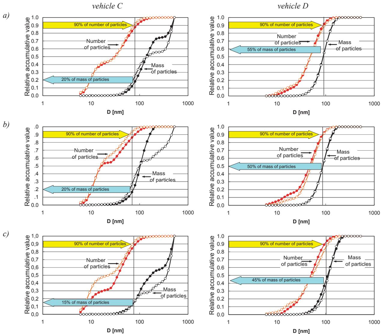
Fig. 11. Relative accumulated value of the PM number and mass as a function of its size recorded on different road portions for tested vehicles A and B: a) urban, b) extra urban, c) expressway; ● – drive with load, ○ – drive without load
