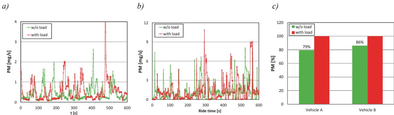
Fig. 4. PM emission rate on the urban road portion: a) vehicle A, b) vehicle B, c) relative values
