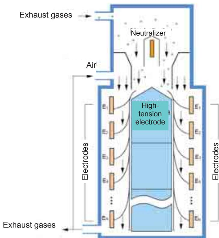
Fig. 2. Schematics of the EEPS 3090 particle sizer
