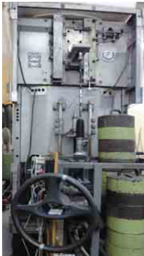
Fig. 6. Measuring stand adapted to input function on the side of the gear-toothed bar. Examined toothed bar is in a vertical position
