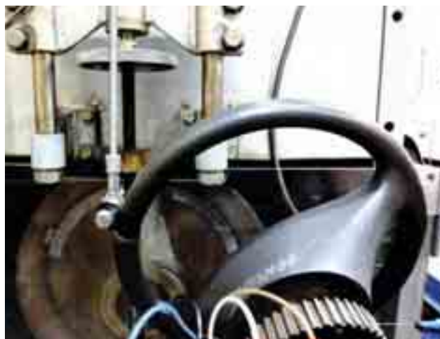
Fig. 4. Measuring stand. View of the mechanical device forcing the steering wheel turning within \pm 500^\circ
