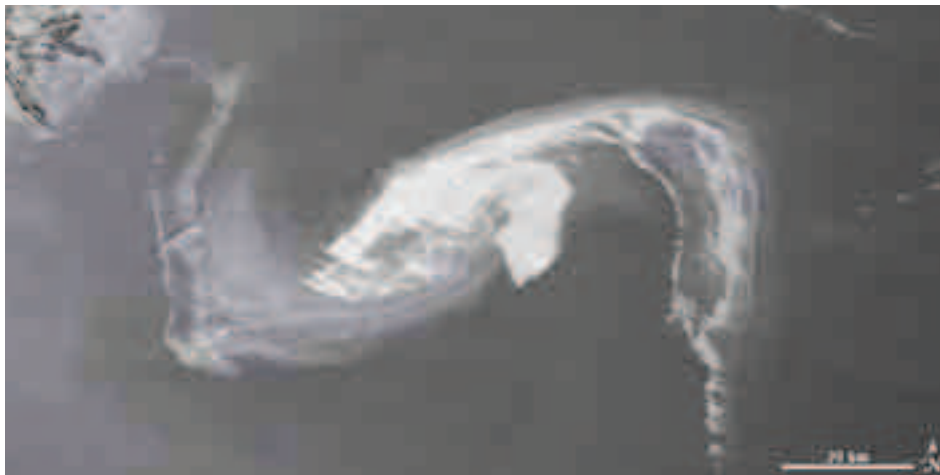
Fig. 1. Image after the process of signals from the satellite Terra (EOS AM-1) equipped by MODIS. There is known that the bright areas show area polluted by crude oil ("Deep Horizon" disaster). There are a lot of oceanic situations (free of oil) in which similar images appear; source: http://commons.wikimedia.org/wiki/File:Gulf_Oil_Spill_Creeps_Towards_Mississippi_Delta_detail_2010-04-29.jpg
