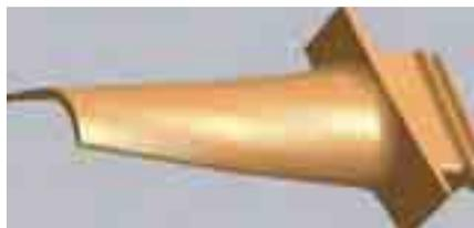
Fig. 1. Model 3D of the engine turbine blades DV - 2
