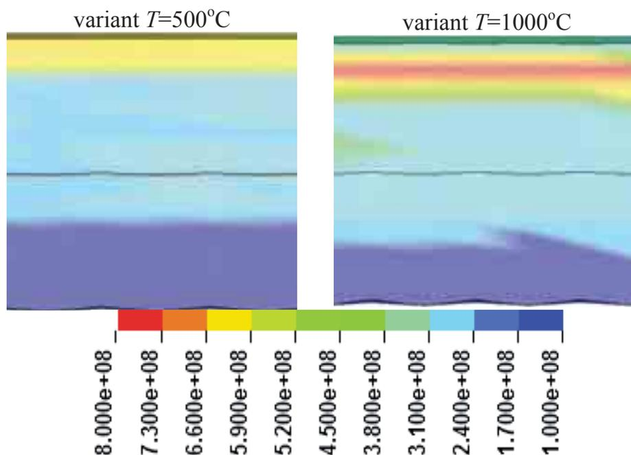
Fig. 5. Maps of the reduced stress (Pa) obtained for  $t = 5 \text{ ms}$  (second model)
