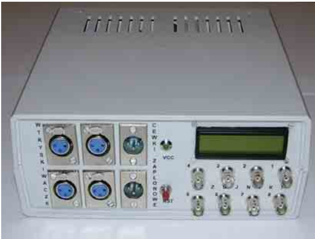
Fig. 2. Controller’s front panel for batched injection
