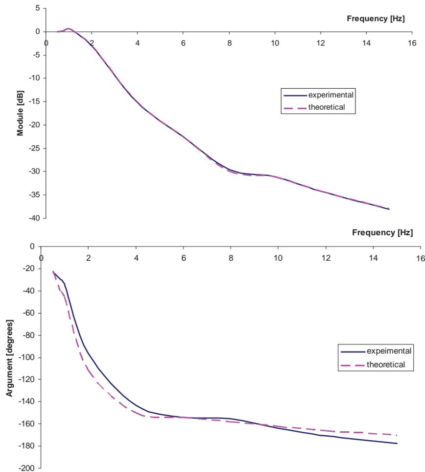
Fig. 3. Theoretical and experimental amplitude-frequency response curves of the investigated hydraulic line for the case (ii), with the transmittance function  $P(l, j\omega) / P(0, j\omega)$
