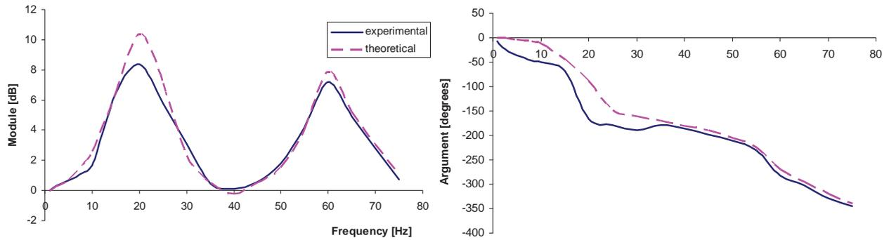
Fig. 6. Theoretical and experimental amplitude-frequency response curves of the investigated hydraulic line for the case (iii), with the transmittance function  $P(0, j\omega) / F(j\omega)$
