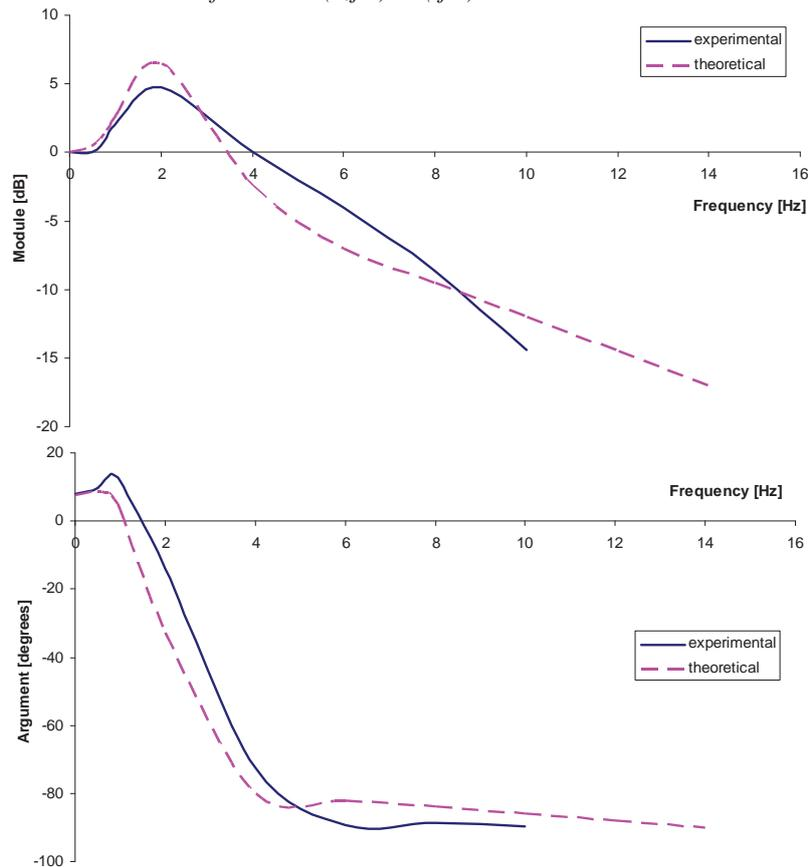
Fig. 7. Theoretical and experimental amplitude-frequency response curves of the investigated hydraulic line for the case (iv), with the transmittance function  $P(l, j\omega) / F(j\omega)$
