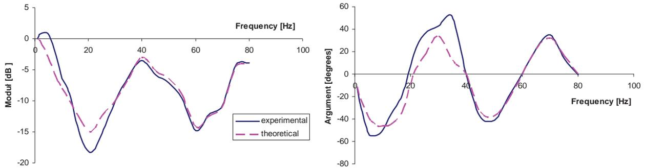
Fig. 2. Theoretical and experimental amplitude-frequency response curves of the investigated hydraulic line for the case (i), with the transmittance function  $P(0, j\omega) / Q(0, j\omega)$
