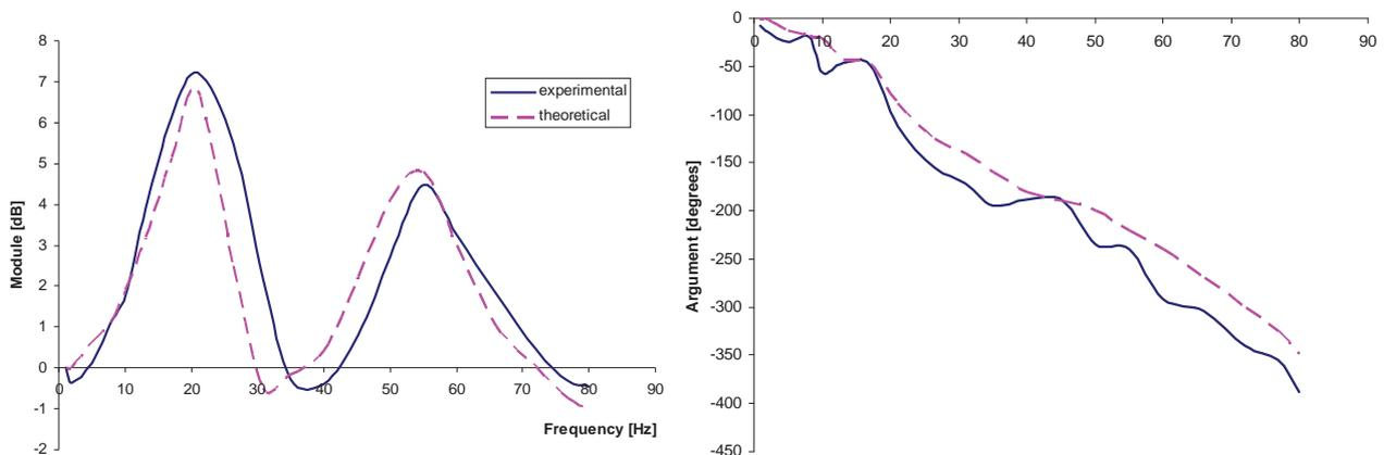
Fig. 1. Theoretical and experimental amplitude-frequency response curves of the investigated hydraulic line for the case (i), with the transmittance function  $P(l, j\omega) / P(0, j\omega)$
