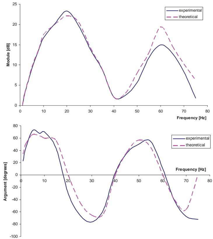
Fig. 5. Theoretical and experimental amplitude-frequency response curves of the investigated hydraulic line for the case (iii), with the transmittance function  $P(l, j\omega) / F(j\omega)$
