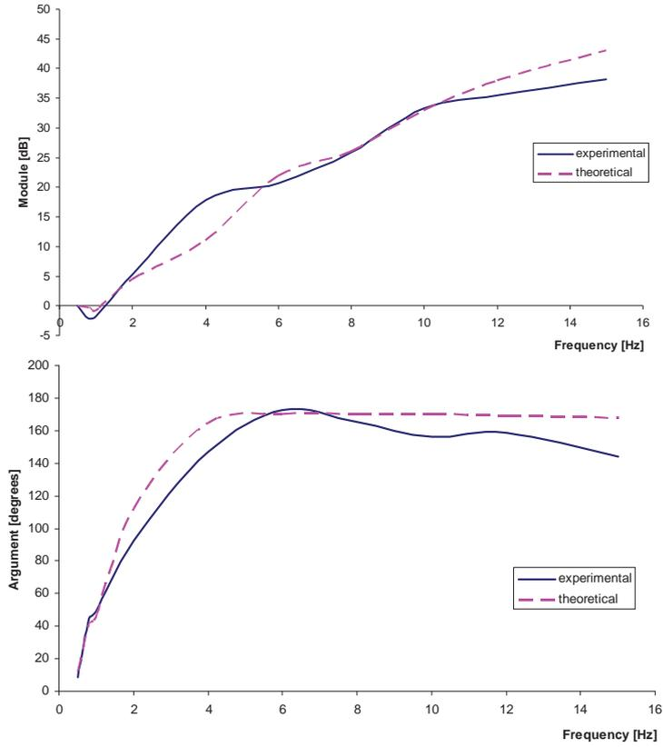
Fig. 4. Theoretical and experimental amplitude-frequency response curves of the investigated hydraulic line for the case (ii), with the transmittance function  $P(0, j\omega) / Q(0, j\omega)$
