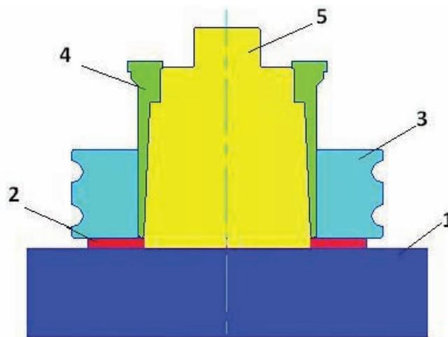
Fig. 6. Shaft, tapered sleeve and carbide ring: 1- Cassette, 2 - Distance ring, 3 - Carbide ring, 4 - Tapered sleeve, 5 - Roll pinion shaft
