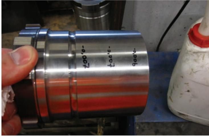
Fig. 7. Tolerances of tapered sleeve's diameter
