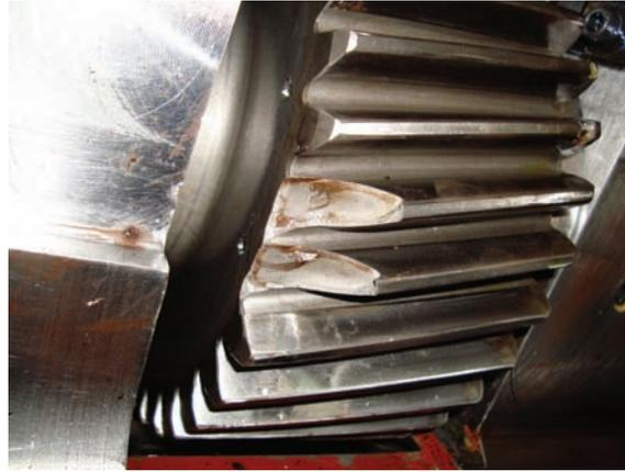
Fig. 3. Broken teeth on the sprocket
