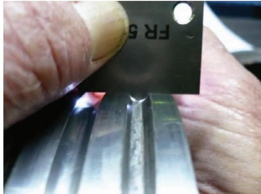
Fig. 9. Checking shape of groove by template
