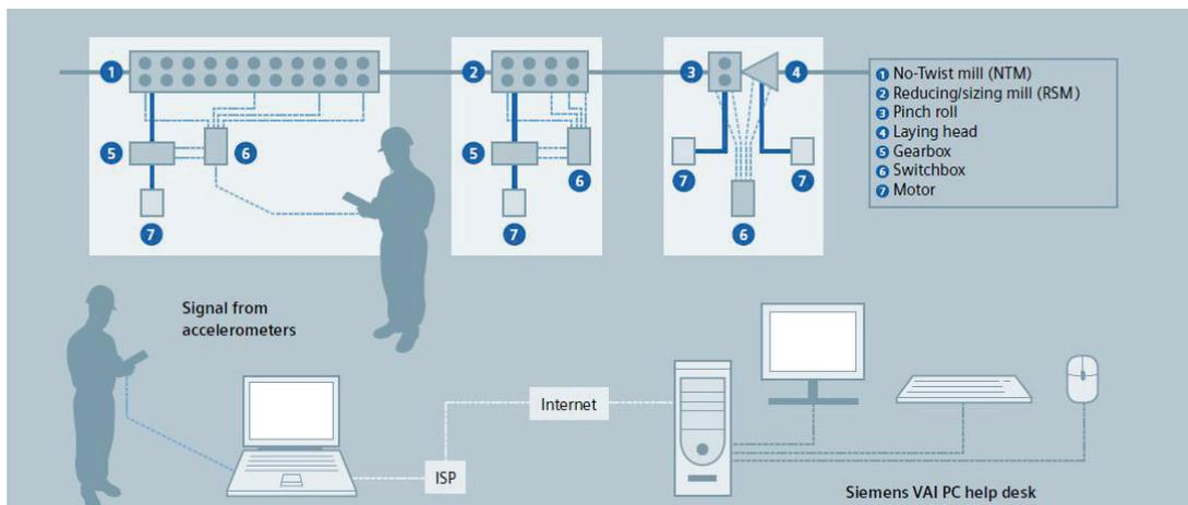
Fig. 4. Measurement of vibrations in Siemens approach [4]
