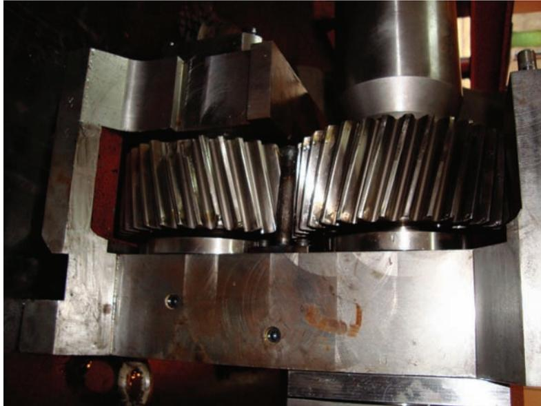
Fig. 5. Destroyed transmission
