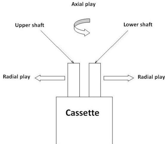
Fig. 1. Control of pinion shaft's clearance
