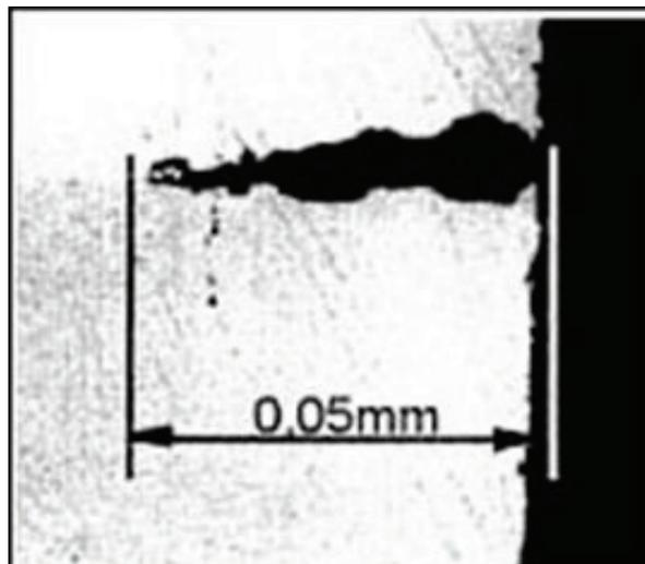
Fig. 12. Micro crack detected with method of eddy current [1]
