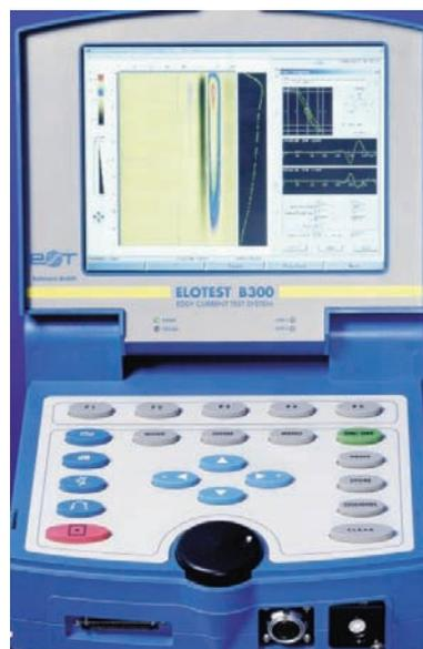
Fig. 10. Eddy current tester for cracks detection [3]
