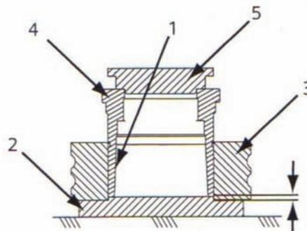
Fig. 8. Pre assembling the taper sleeve and the ring: 1- Surface to use blue ink, 2 - Assembly plate, 3 - Carbide ring, 4 - Tapered sleeve, 5 - Press side
