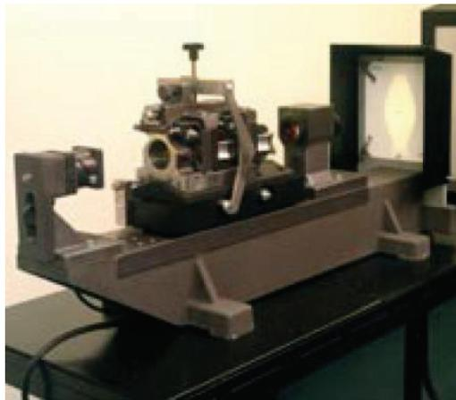
Fig. 15. Optical device for checking guide assembly [2]
