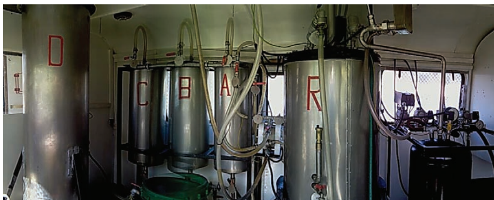
Fig. 4. A panoramic photograph of a mobile diesel production plant, built on a chassis of a Star 266 vehicle. The transesterification reactor(R) with the post-reaction mixture separators (A, B, C)
