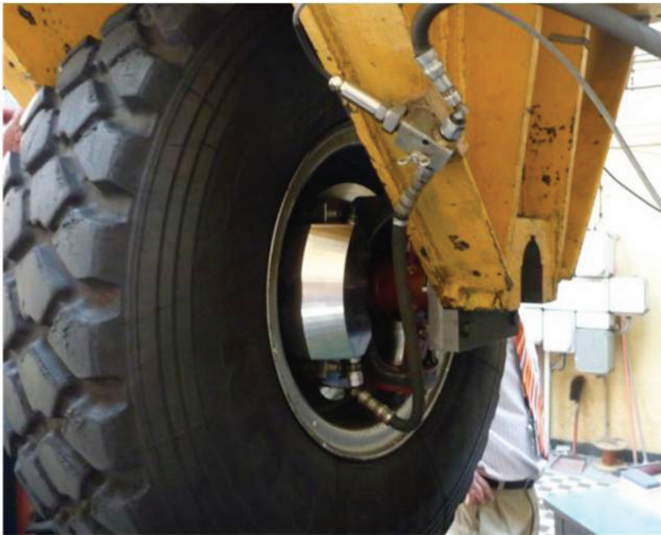
Fig. 7. 3 piston brake mounted to the test stand
