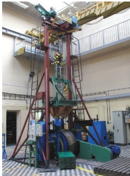
Fig. 2. Drop test machine used in brake testing
