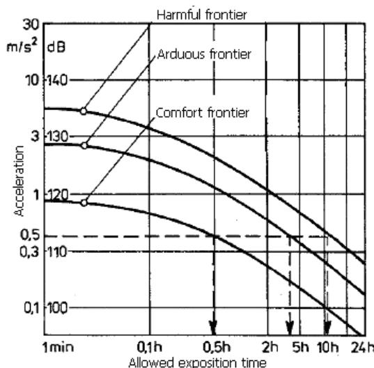
Fig. 1. Allowable acceleration values [3]
