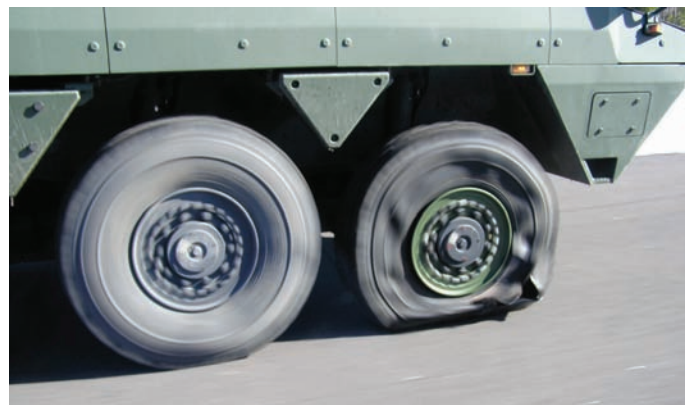
Fig. 2. Experimental studies of the vehicle with a damaged tire
