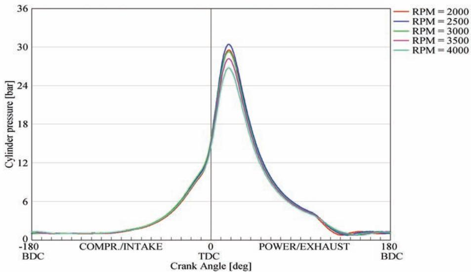
Fig. 3. Courses of cylinder pressure at different rotational speeds
