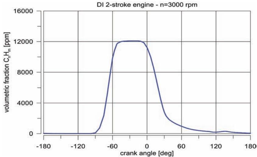
Fig. 2. Volumetric fraction of gaseous fuel ( $C_nH_m$ ) in cylinder of 2-stroke engine DFI 125 cc at WOT and 3000 rpm
