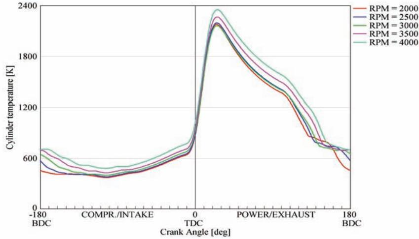
Fig. 4. Courses of cylinder temperature at different rotational speeds
