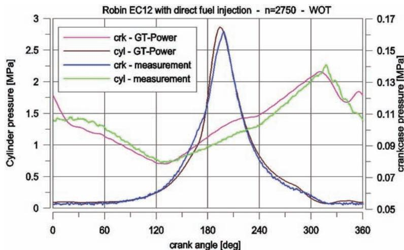
Fig. 7. Comparison of calculated and measured pressure in cylinder and crankcase
