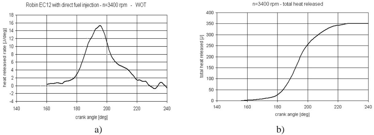
Fig. 8. a) Heat release rate at 3400 rpm and b) total heat released at 3400 rpm and full load
