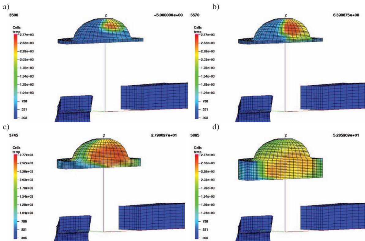
Fig. 1. Distribution of temperature in DFI two-stroke engine at 3000 rpm and at piston position: a) 5 deg CA BTDC, b) 6.3 deg CA ATDC, c) 27.9 deg CA ATDC and d) 53 deg CA ATDC
