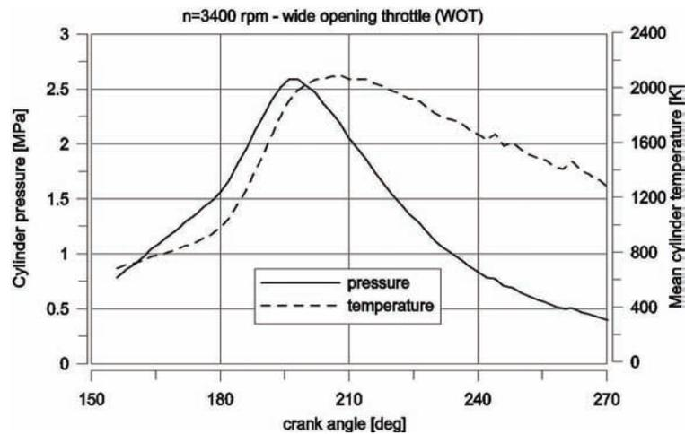
Fig. 6. Cylinder temperature and pressure during combustion process at 3400 rpm
