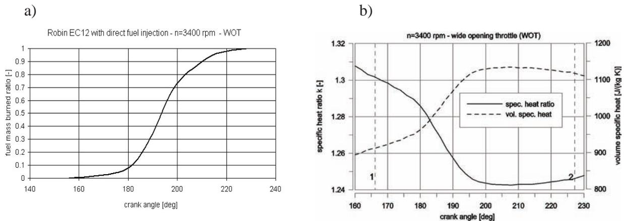
Fig. 10. a) Variation of fuel mass burned ratio at 3400 rpm, b) variations of specific heat at constant volume and specific heat ratio during combustion process at 3400 rpm
