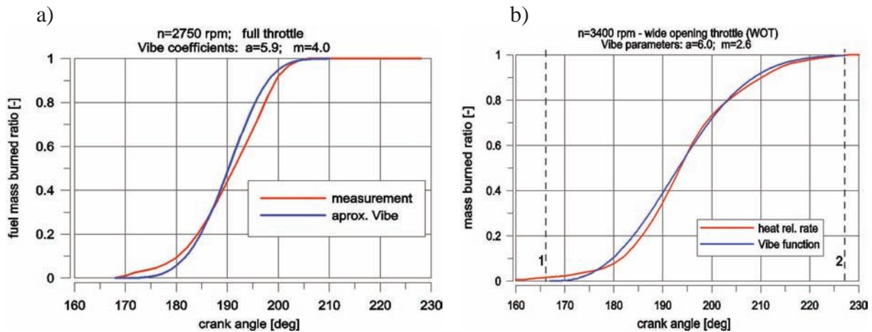
Fig. 10. Fuel mass burned ratio and approximated Vibe function in combustion process at a) 2750 rpm, b) 3400 rpm
