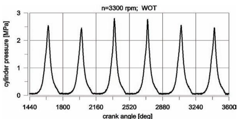
Fig. 5. Inequality of pressure in engine with direct fuel injection at 3300 rpm 50% WOT
