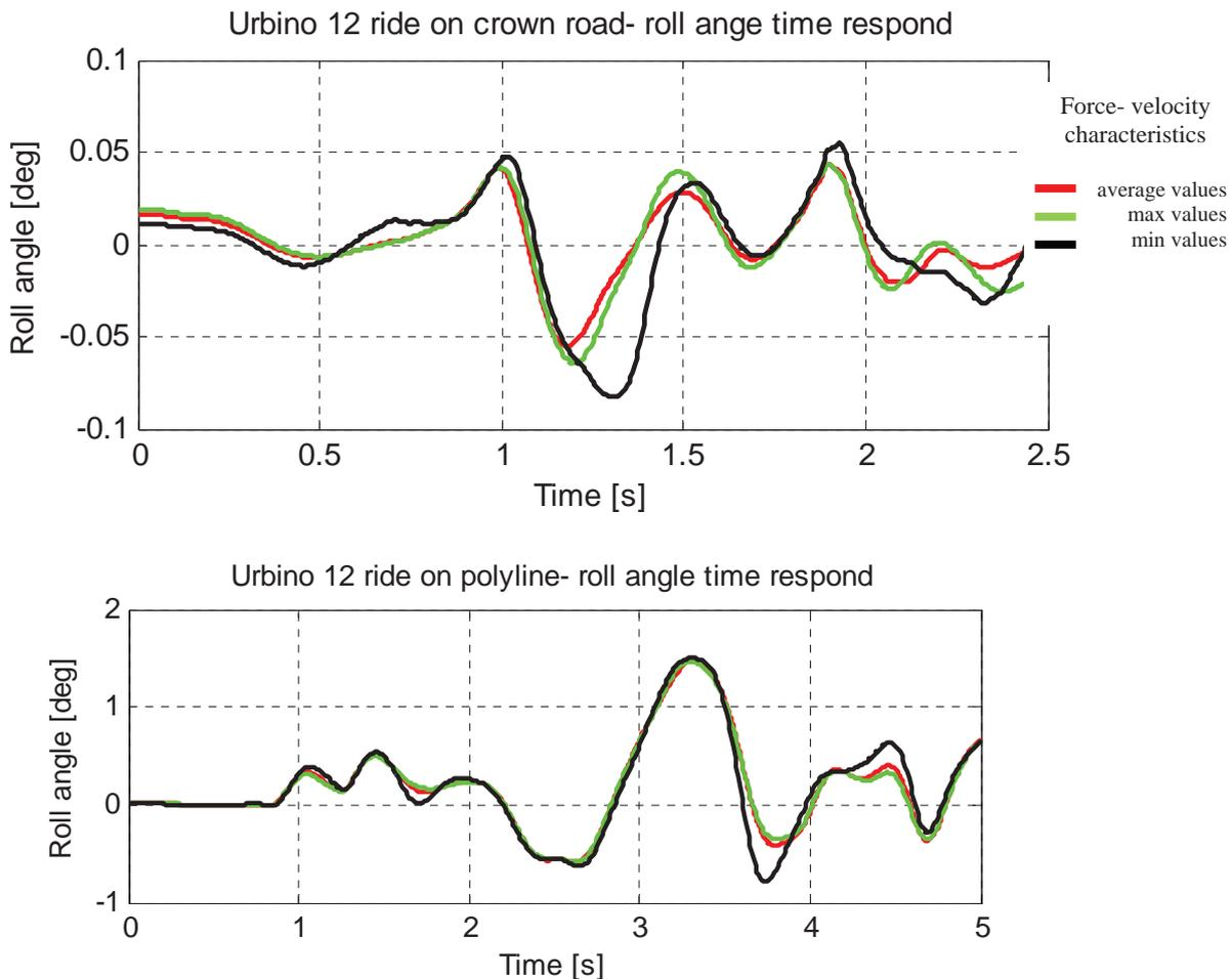
Fig. 5. Roll angle time respond with tree different force-velocity characteristics of damper element while riding on two different road profiles (crown upper one and polyline lower one)
