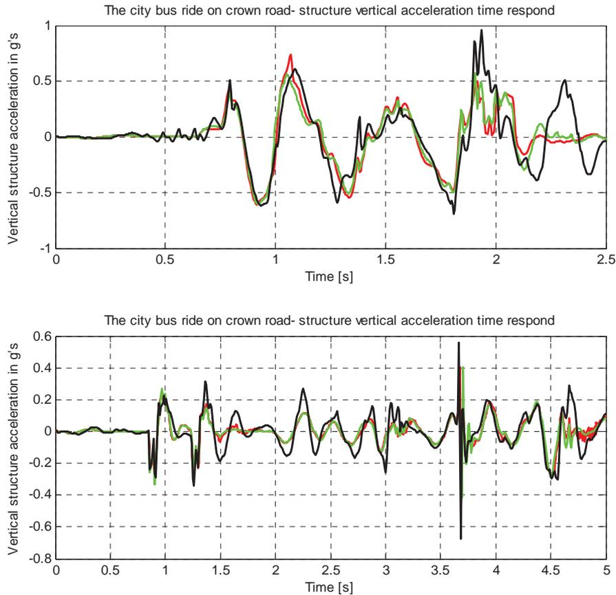
Fig. 7. Structure vibration accelerations time respond with three different force-velocity characteristics of damper element while riding on two different road profiles (crown upper one and polyline lower one)
