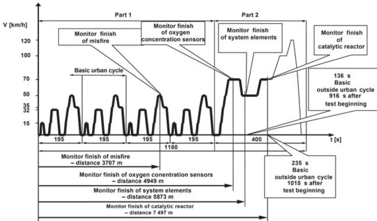
Fig. 1. Monitor realization of the NEDC test in temperature +22°C
