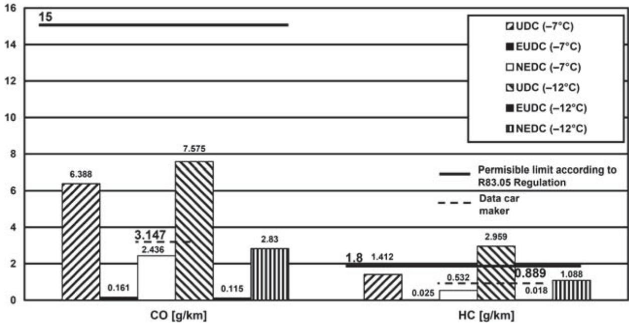
Fig.4. Road emissions of a car during the NEDC (UDC + EUDC) European drive cycle in low temperature chamber (-7°C) in comparison to emissions in temperature -12°C
