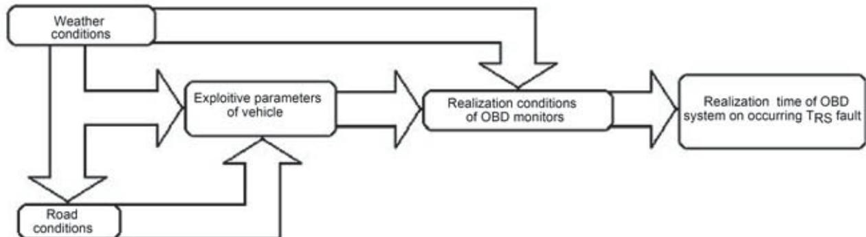
Fig. 9. Relations between parameters influencing on OBD system reaction time for defect appearing
