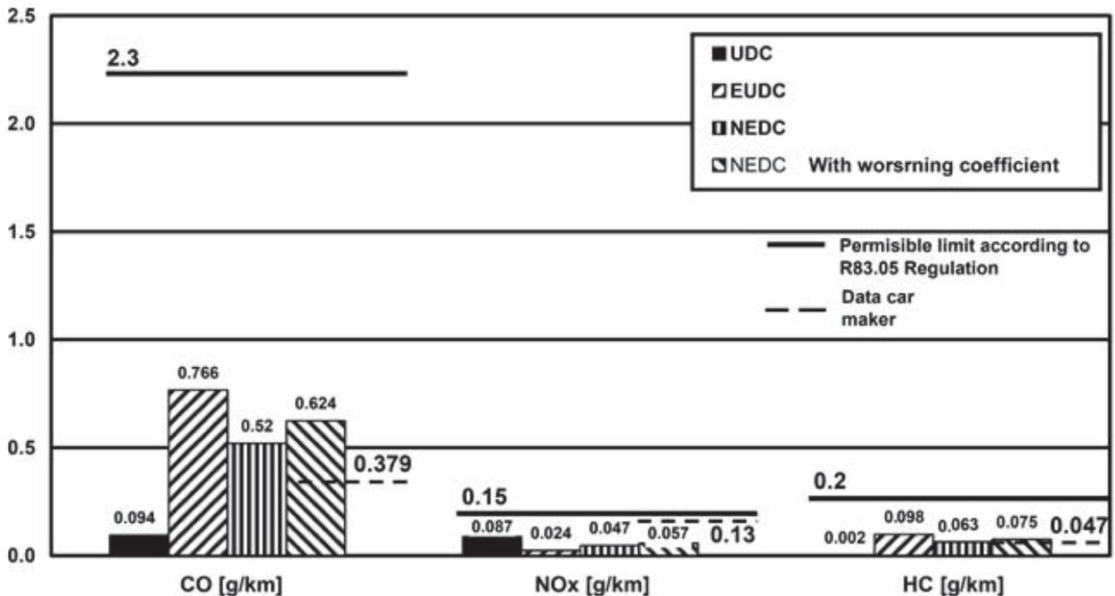
Fig. 3. Road emissions of a car during the NEDC (UDC + EUDC) European drive cycle
