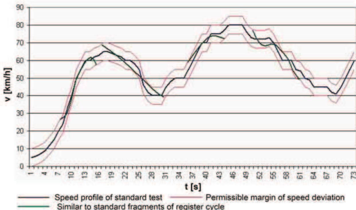
Fig. 7. Comparison idea of road cycle piece with pattern cycle similar from point of view speed course
