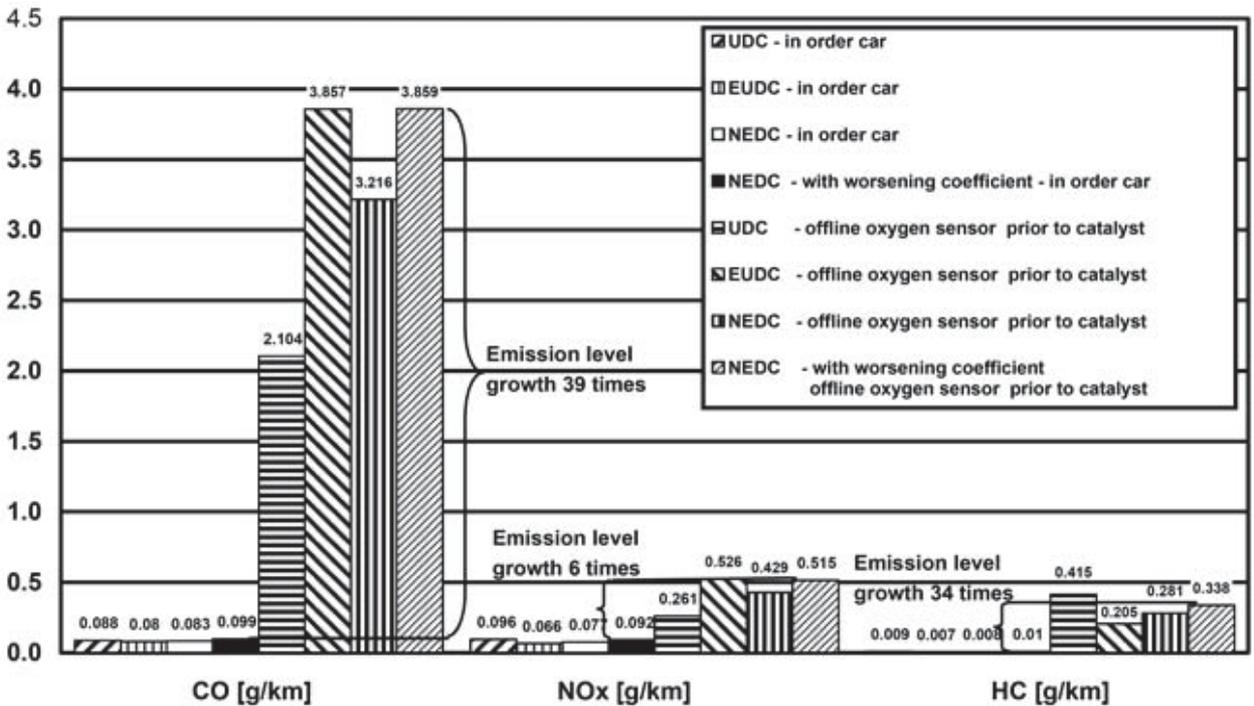
Fig. 5 Road emissions of a car during the European drive cycle in comparison to emissions at oxygen sensor disconnected before catalytic reactor
