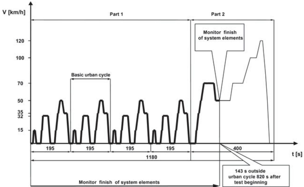
Fig. 2. Monitor realization of the NEDC test in temperature  $-12^{\circ}\text{C}$
