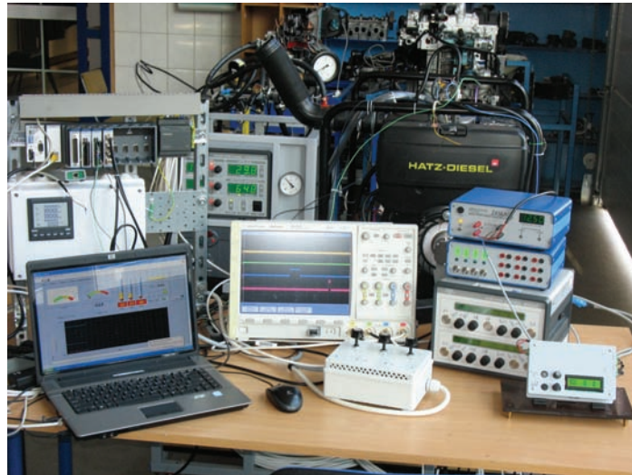
Fig. 3. A view of a HATZ 1B40 engine with a system for controlling, monitoring and fuelling with CNG and diesel oil
