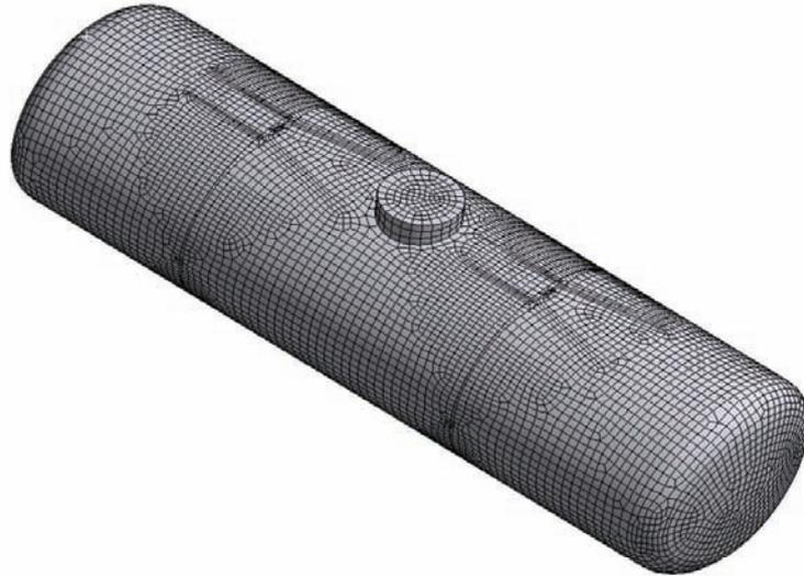
Fig. 2. CFD model of the tank, 3D hexahedral cells
