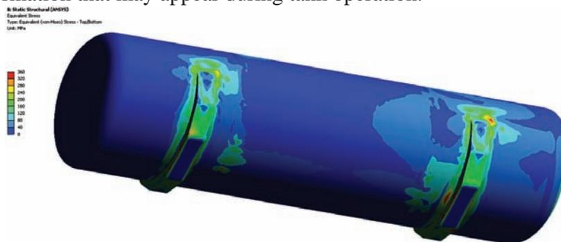
Fig. 7. FEA results, equivalent stress [N/mm<sup>2</sup>]
