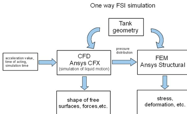
Fig. 4. One way FSI simulation of the tank
