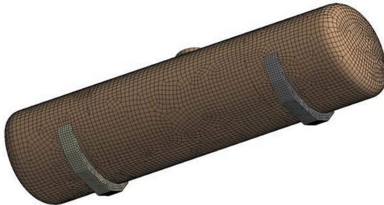
Fig. 3. FEA model of the tank, quadrilateral shell elements
