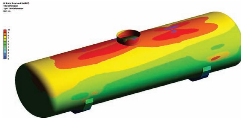
Fig. 8. FEA results, total displacement [ mm]
