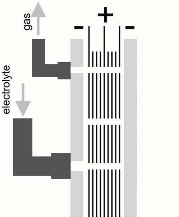
Fig. 3. Scheme of Brown gas generator
