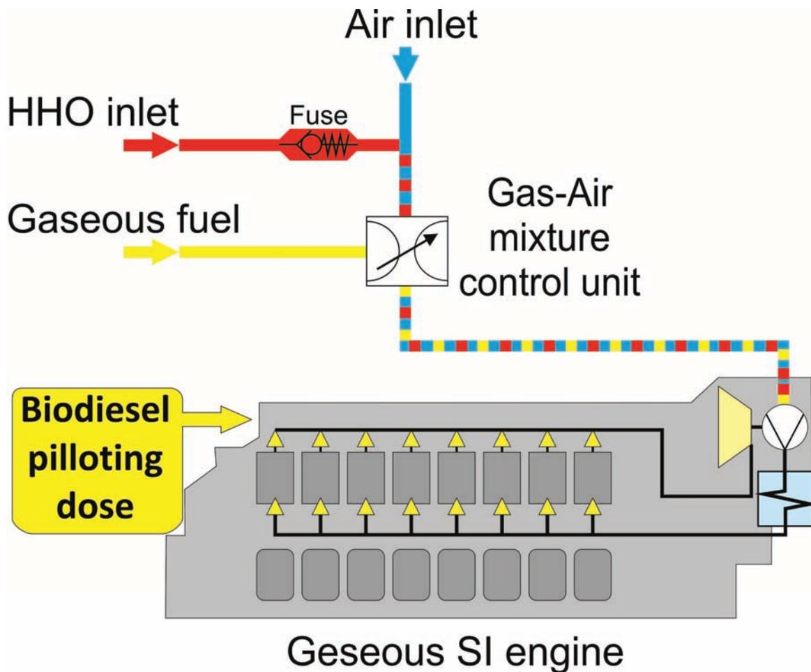
*Fig. 2. Diagram of connection generator to the engine when the gas is feed to inlet manifold*
