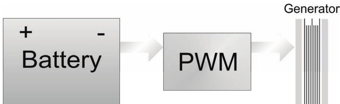
Fig. 5. Diagram of power supply system of gas generator
