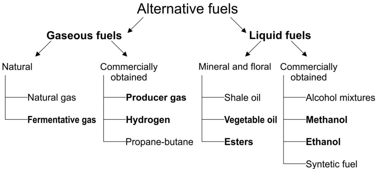
Fig. 1. Division of alternative fuels used to power internal combustion engines [2]
