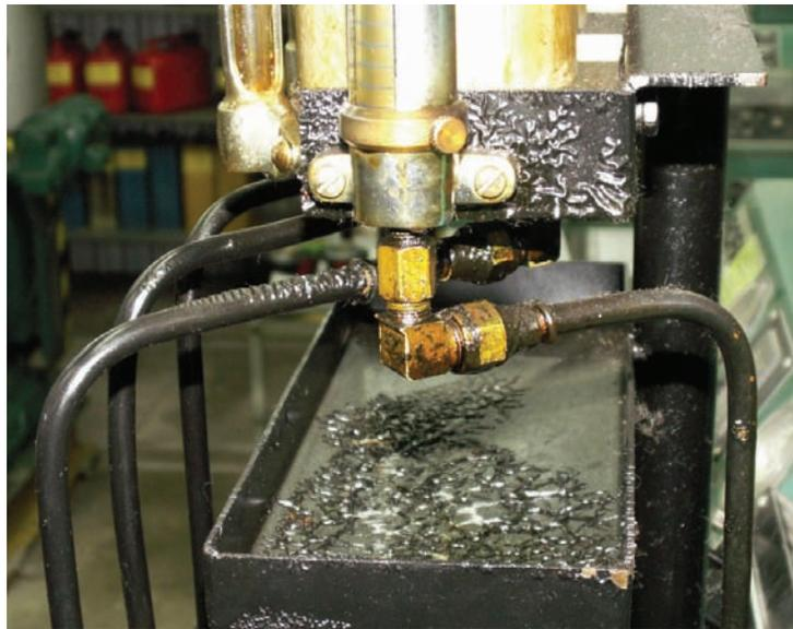
Fig. 6. Biofuels influence on fuel pipes protective coating of CFR Waukesha test engine for Cetane number determination (O&GI Cracow)
