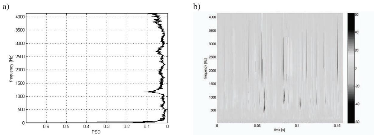
Fig.5.I. The results obtained for shift of a cog belt by two teeth : a) – frequency distribution of power spectrum density of the vibration acceleration signal, b) - time-frequency distribution of wavelet coefficients, view 2D
