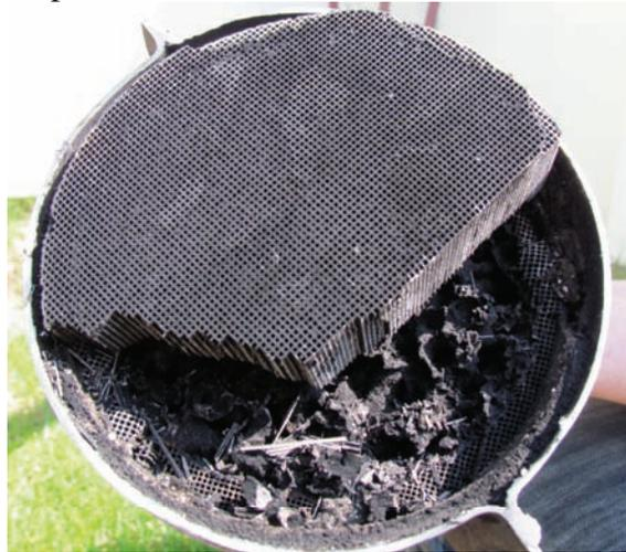
Fig. 1. The catalytic converter damage caused by overheating
