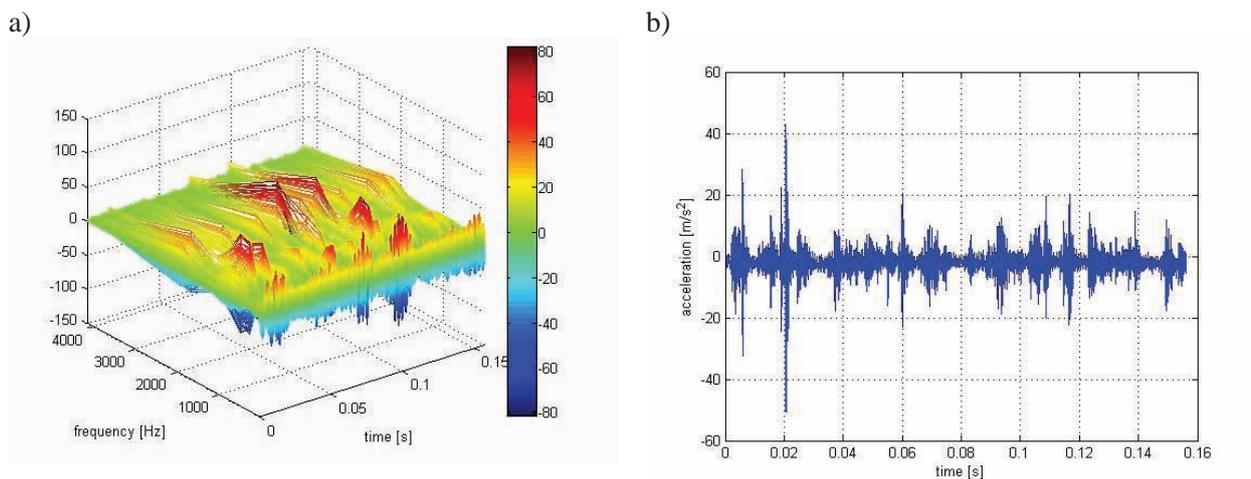
Fig. 4. II. The results obtained for shift of a cog belt by one tooth a) – 3D wavelet distribution of vibration acceleration in a selected frequency band, b) – fragment of the analysed signal
