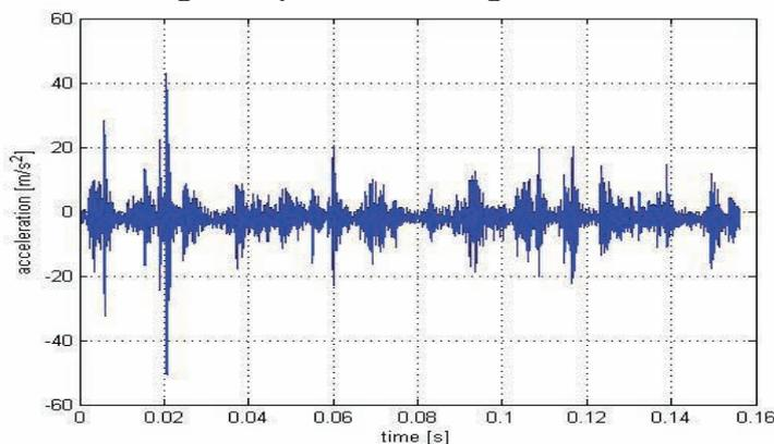
Fig. 2. Part of vibration acceleration signal recorded upon the engine case at half height of the first cylinder
