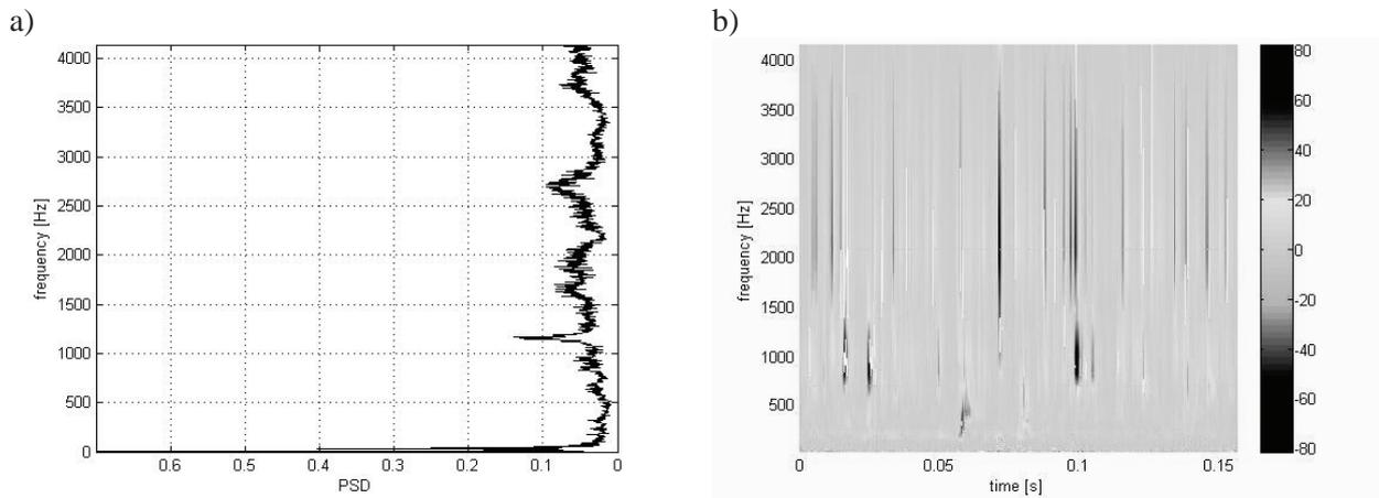
Fig. 4. I. The results obtained for shift of a cog belt by one tooth a) – frequency distribution of power spectrum density of the vibration acceleration signal, b) - time-frequency distribution of wavelet coefficients ,view 2D
