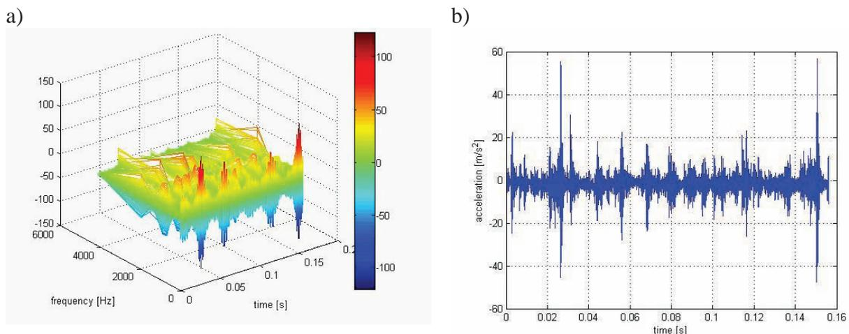
Fig. 3. II. The results obtained for the engine in nominal technical conditions: a) – 3D wavelet distribution of vibration acceleration in a selected frequency band, b) – fragment of the analysed signal
