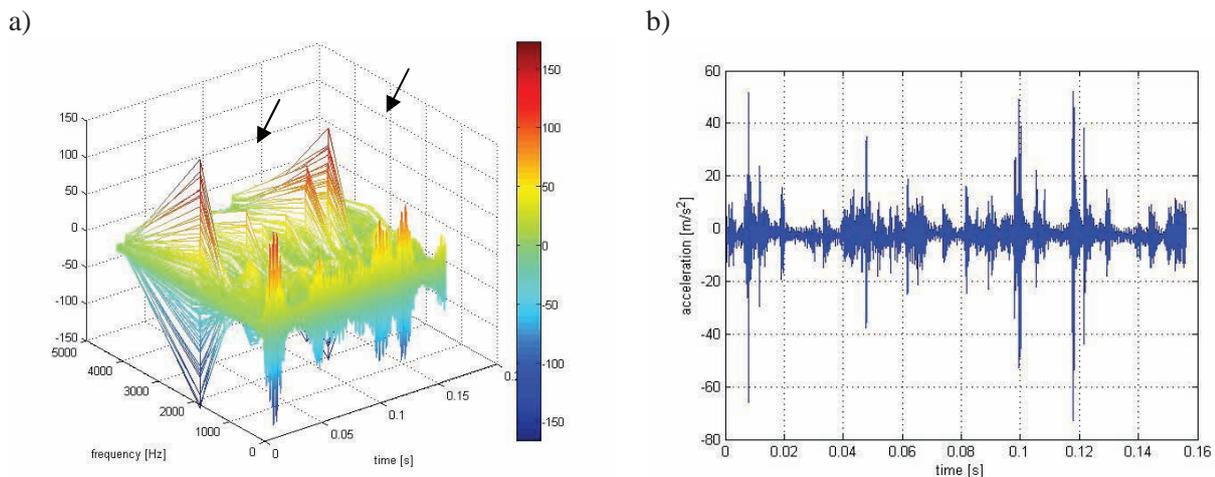
Fig. 7. II. The results obtained at the reduced surface area of the exhaust channel cross section by 85%: a) – 3D wavelet distribution of vibration acceleration in a selected frequency band, b) – fragment of the analysed signal
