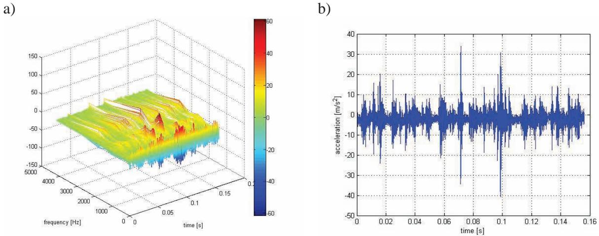
Fig. 5. II. The results obtained for shift of a cog belt by two teeth: a) – 3D wavelet distribution of vibration acceleration in a selected frequency band, b) – fragment of the analysed signal
