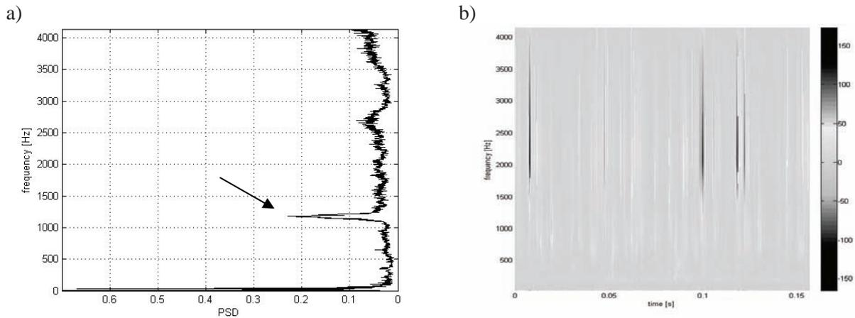
Fig. 7. I. The results obtained at the reduced surface area of the exhaust channel cross section by 85%: a) – frequency distribution of power spectrum density of the vibration acceleration signal, b) - time-frequency distribution of wavelet coefficients, view 2D
