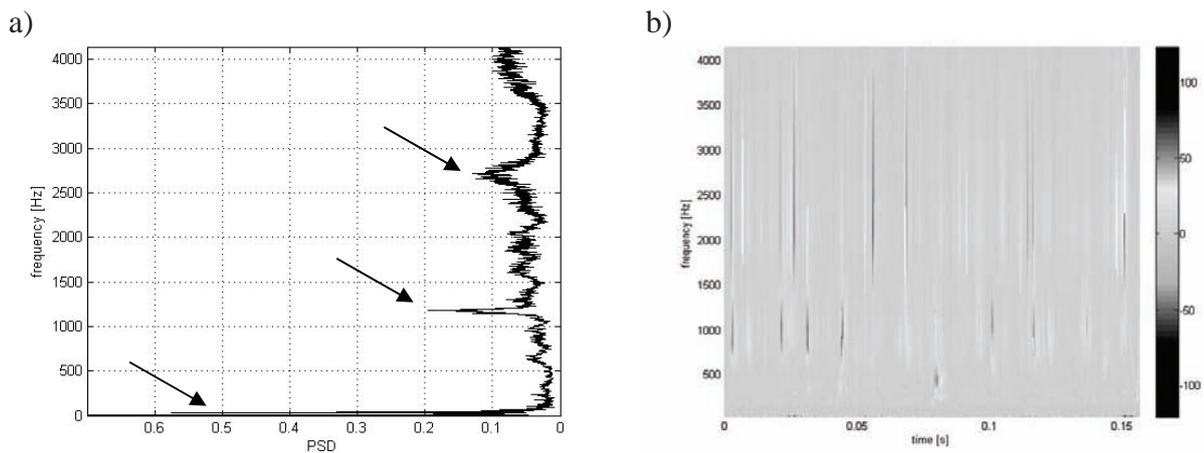
Fig. 3. I. The results obtained for the engine in nominal technical conditions: a) – frequency distribution of power spectrum density of the vibration acceleration signal, b) - time-frequency distribution of wavelet coefficients ,view 2D
