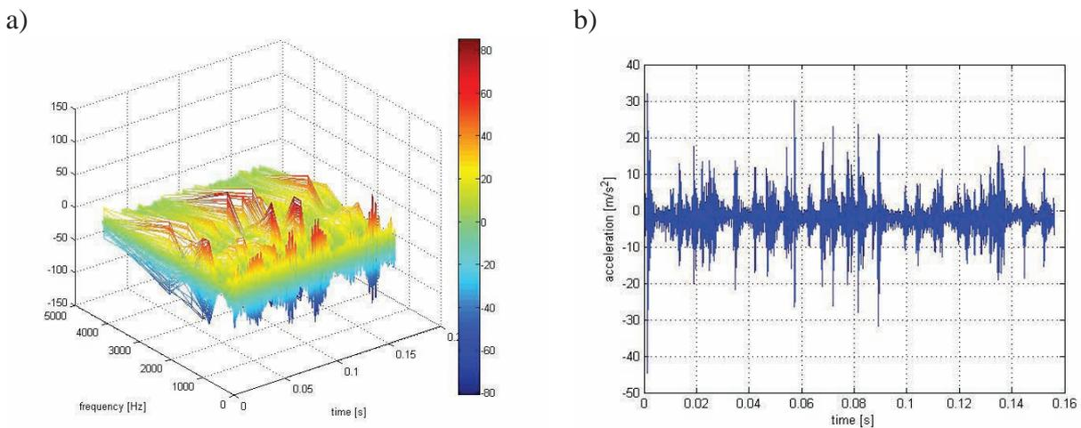
Fig. 6. II. The results obtained at the reduced surface area of the exhaust channel cross section by 75%: a) – 3D wavelet distribution of vibration acceleration in a selected frequency band, b) – fragment of the analysed signal
