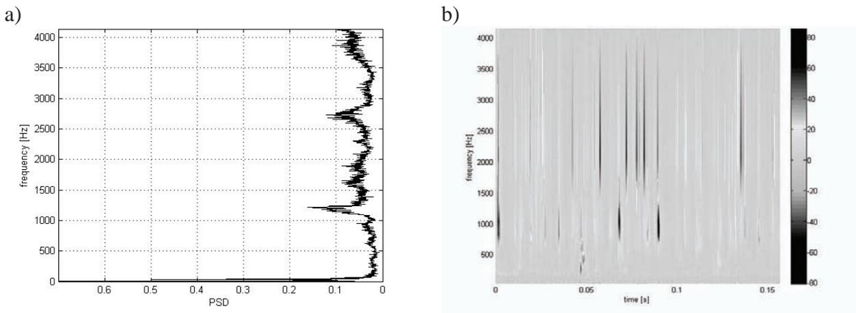
Fig. 6. I. The results obtained at the reduced surface area of the exhaust channel cross section by 75%: a) – frequency distribution of power spectrum density of the vibration acceleration signal, b) - time-frequency distribution of wavelet coefficients, view 2D
