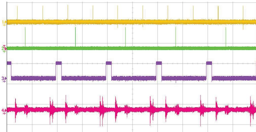
Fig. 2. Example oscilloscope trace of time courses of signals reflecting: - crankshaft position (channel 1), - top dead center piston position between the compression and working strokes (channel 2), - determined level of intake valve opening (channel 3), - vibration accelerations (channel 4); for a HATZ 1B40 engine operating at 3000 rpm; Time base scale: 20 ms per division. Vibration signal value scale: 2 V per division
