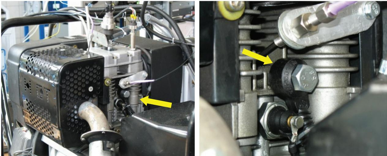
Fig. 3. Location of mounting of the vibration acceleration sensor on the engine (the sensor is indicated with the yellow arrow)
