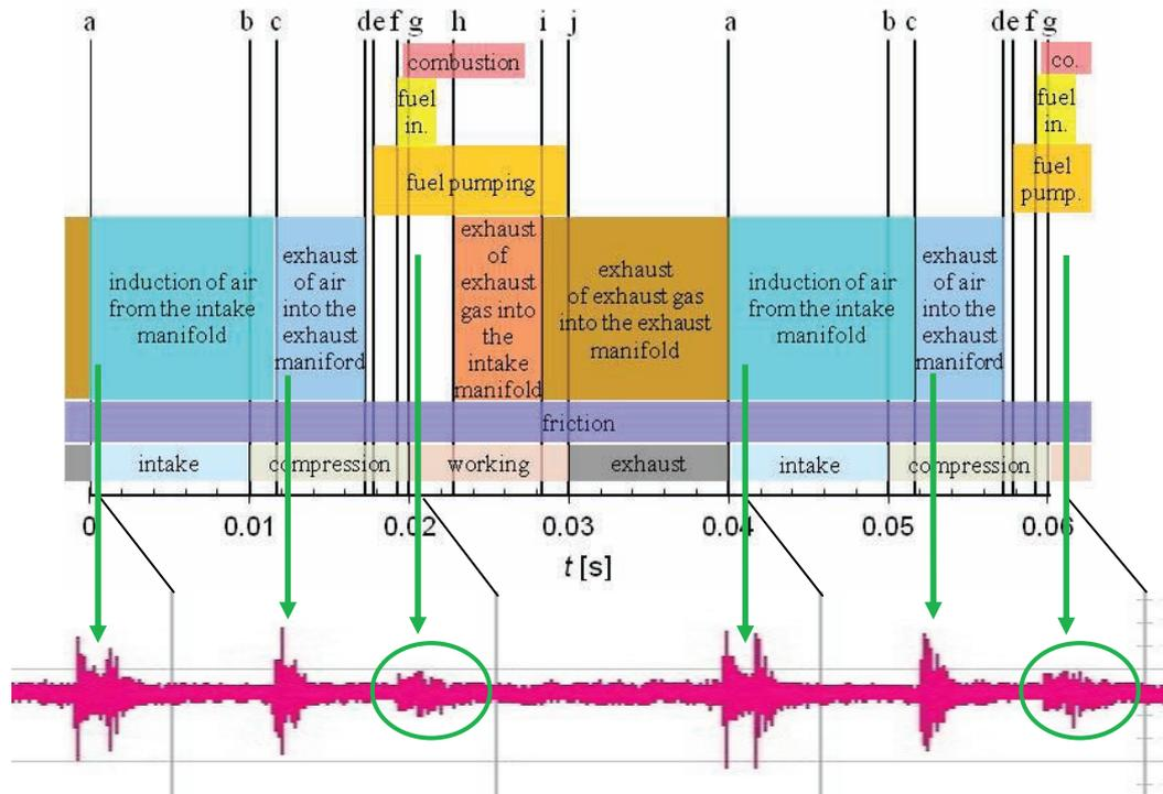
Fig. 4. Allocation of the theoretical (top) and empirical (bottom) time course of the vibration signal of the HATZ 1B40 engine for crankshaft speed of 3000 rpm with marked with ovals fragments corresponding to diesel oil injection, its spontaneous ignition and start of air-fuel mixture combustion
