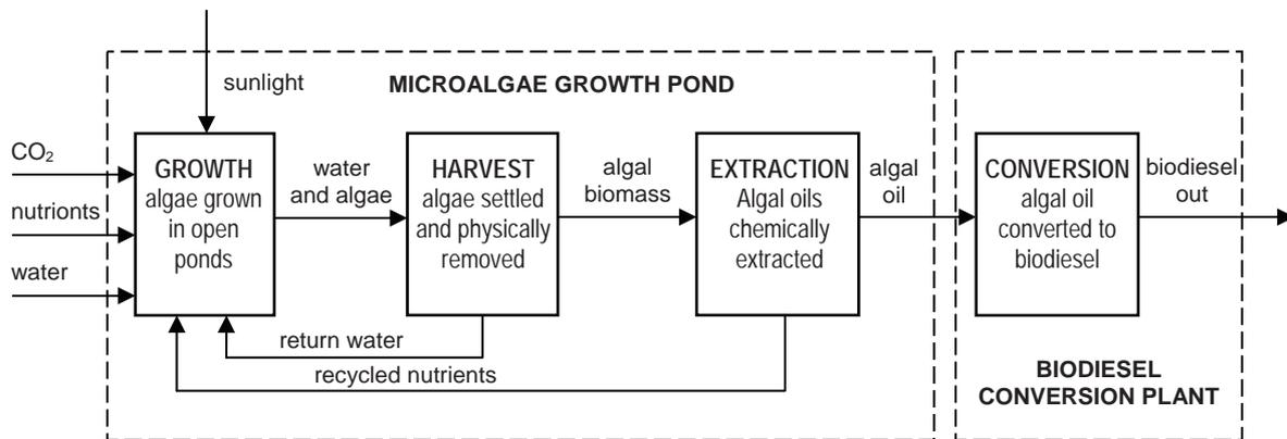
Fig. 4. Simplified systems block diagram of the algae to biodiesel process [4]
