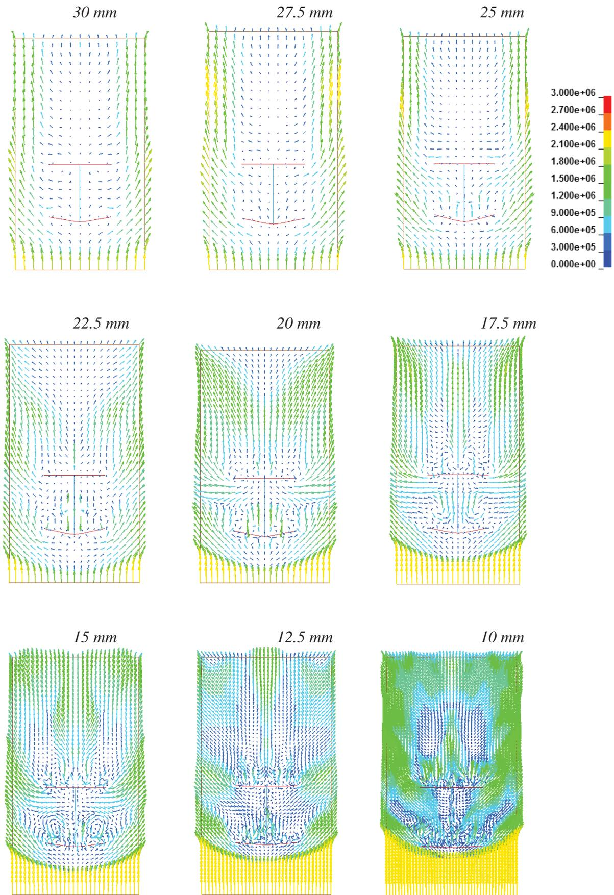
Fig. 8. Velocity vectors at 0.001 s [mm/s]
