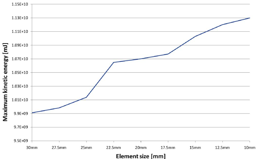
Fig. 6. Maximum Eulerian domain kinetic energy vs. element size
