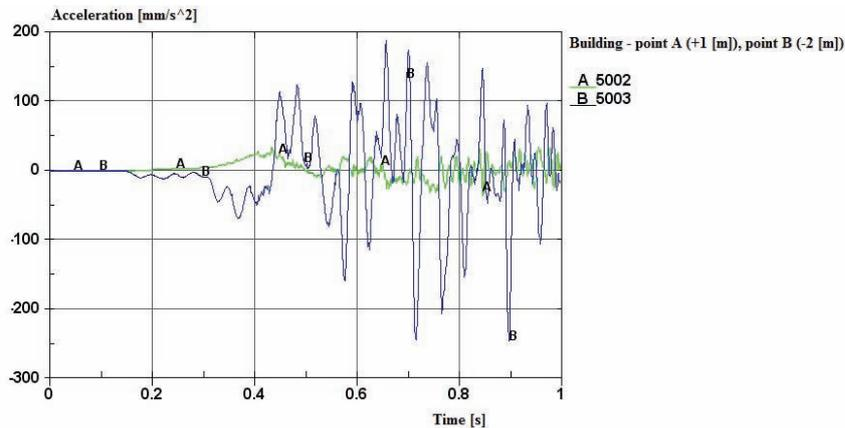
Fig. 11. Amplitude of the vibration acceleration of the foundation of the building in the Y direction
