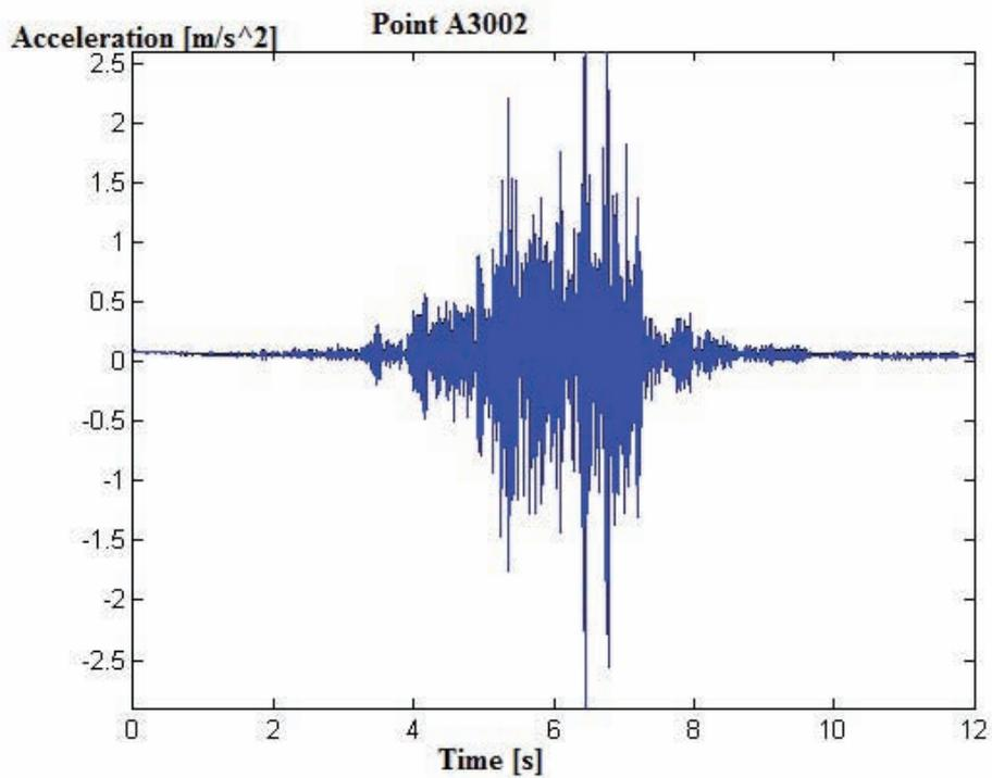
Fig. 9. Amplitude of vibration acceleration of soil vibrations at the measuring point 2 measured during the experiment
