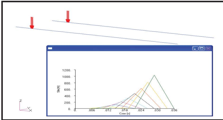
Fig. 5. Example of the amplitude of force for several track nodes
