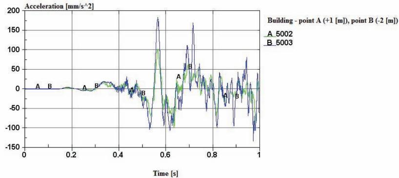
Fig. 10. Amplitude of the vibration acceleration of the foundation of the building in the X direction
