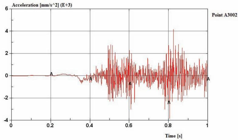
Fig. 8. Amplitude of vibration acceleration of soil vibrations at the measuring point 2 obtained from simulations
