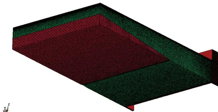
Fig. 4. Boundary conditions of FEM model
