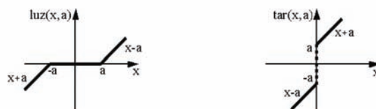
Fig. 2. Topology of luz(\dots) and tar(\dots) projections
