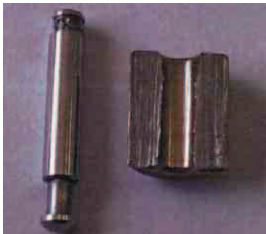
Fig. 2. The view of measured non used and non damaged surfaces with longitudinal nano-ridges and grooves in cylindrical slide microbearing journal and sleeve, for computer ventilator Xilence Case Fan Flow
