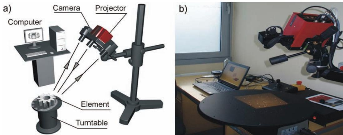
Fig. 1. The measuring system GOM ATOS: a) schema, b) photography
