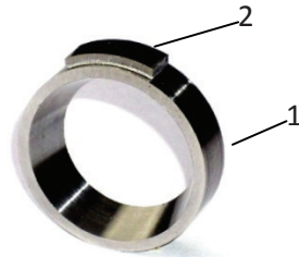
Fig. 1. The sliding pair; 1-ring sample, 2-counter-sample
