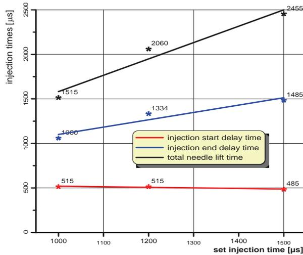
Fig. 4. Total needle lift times, delay of the start and end of the one-part injection depending on the set injection time
