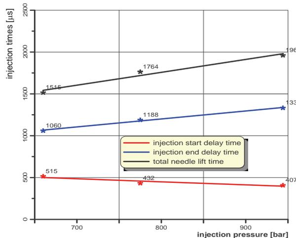
Fig. 5. Total needle lift times, delay of the start and end of the one-part injection depending on the injection pressure
