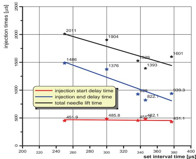
Fig. 6. Total needle lift times, delay of the start and end of the injection for the two-part dose depending on the set interval time
