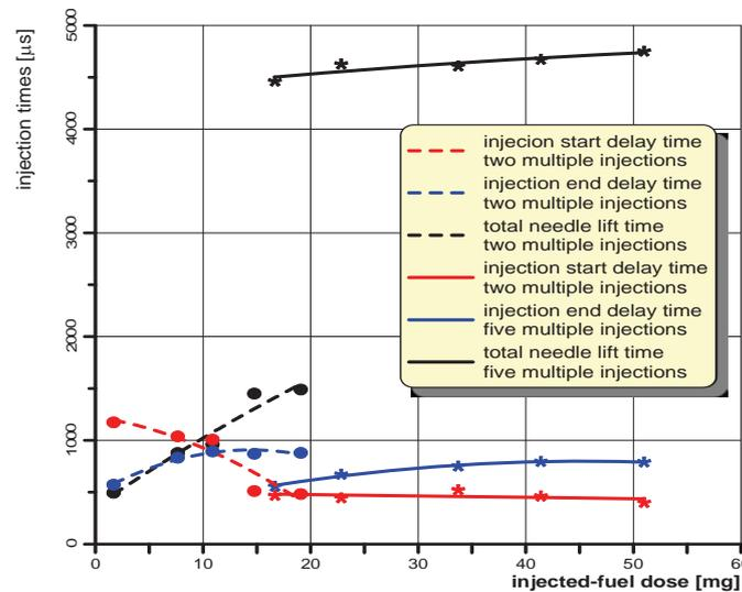
Fig. 2. The delay of the injection start and end depending on fuel dose
