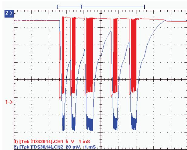
Fig. 3. Courses of injector control voltage and current for division of the dose into five parts
