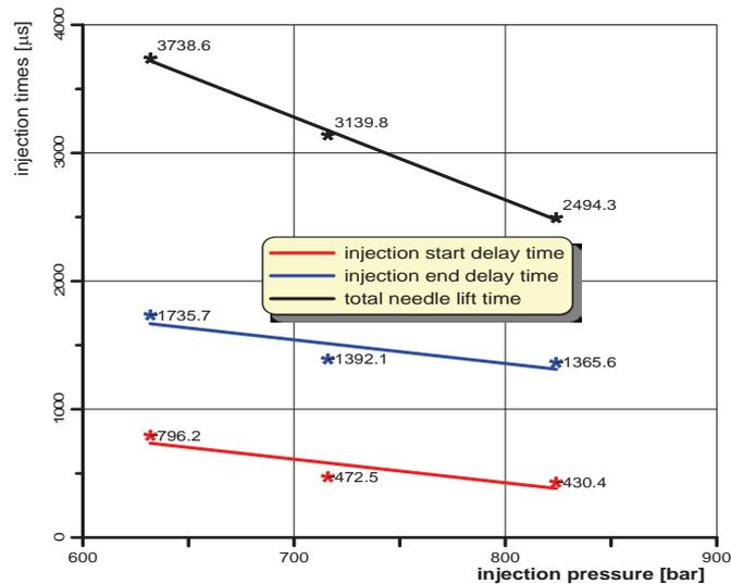
Fig. 7. Total needle lift times, delay of the start and end of the injection for the two-part dose depending on pressure in the accumulator for the second group of measurements
