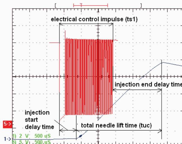
Fig. 1. Measured courses: injector control course (red line) and pressure in the indicator chamber (blue line) with characteristic injection times marked
