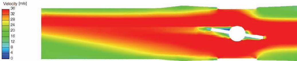
Fig. 13. Velocity distribution in the throttle cross-section for the angle of  $80^\circ$
