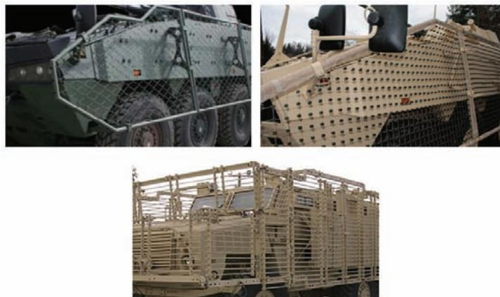
Fig. 1. Type of the applied net and bar screens
