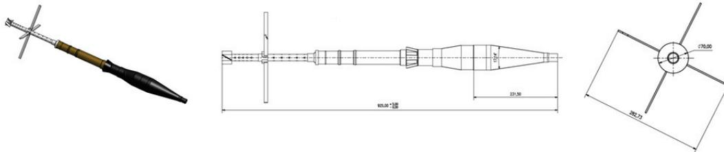
*Fig. 3. PG-7M grenade diagram*
