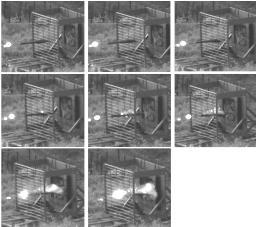
Fig. 2. Destruction of the grenade on the bar screen. Exemplary shots from the high speed camera
