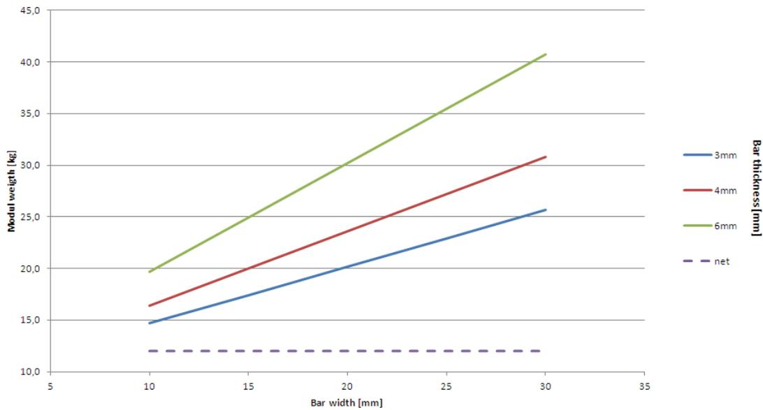
Fig. 8. the change of 1500x1000 module weight for the selected net and bar screen
