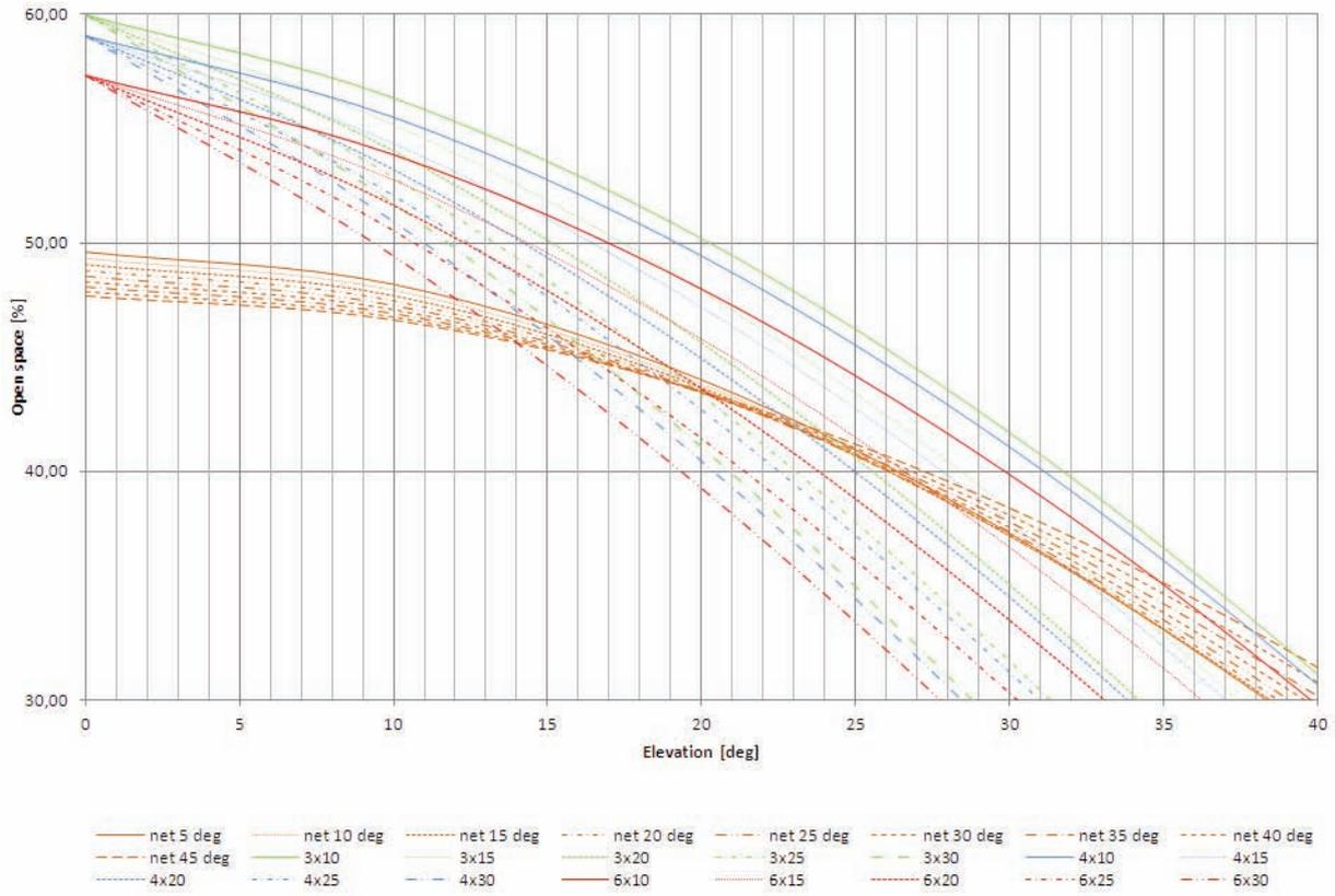
Fig. 6. The changes in the open space depending on changes in grenade impact angle in elevation
