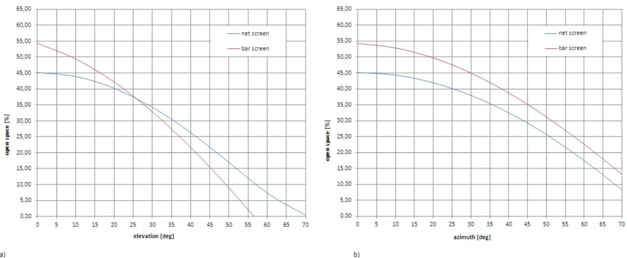
Fig. 9. The comparison of the selected bar screen (red line) and net screen (blue line). The function of the open space (calculated in percentage) on angles in a) elevation, b) azimuth
