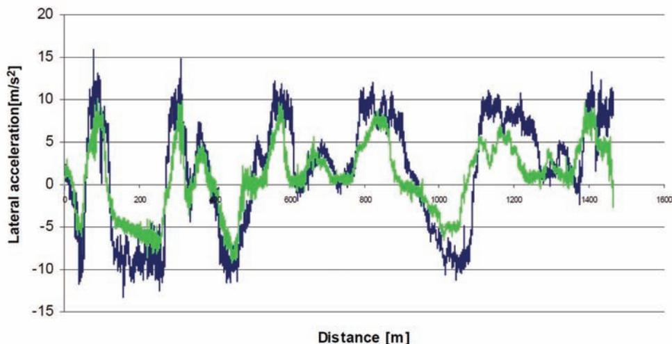
Fig. 6. Characteristics of lateral acceleration affecting the car in the function of the path for the fastest and slowest driver in the test (blue fast driver, green slow)
