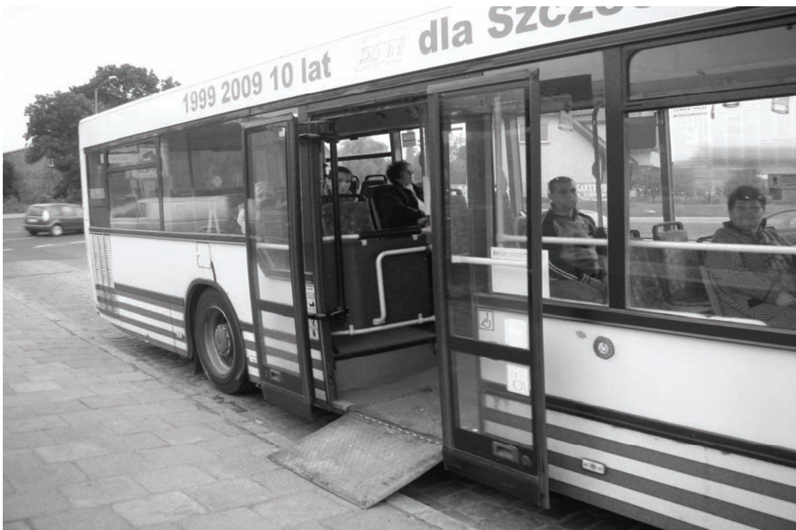
Fig. 1. MAN NL262 bus of the Szczecin Bus Company "Dąbie" (SPAD) performing a kneeling system operation by unfolded manually-operated ramp
