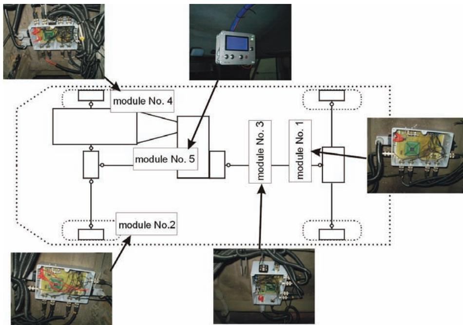
Fig. 3. Location of actuating modules in the Tarpan Honker vehicle
