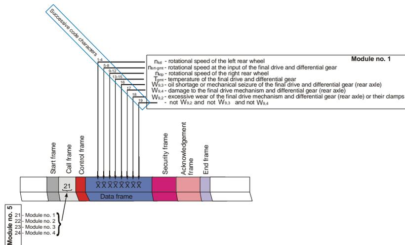
Fig. 2. Principal structure of the data protocol generated by module No. 1
