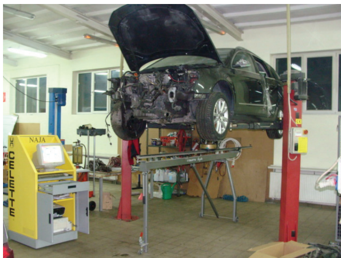
Fig. 7. The investigation of VW Passat car body with the use of NAJA measuring system
