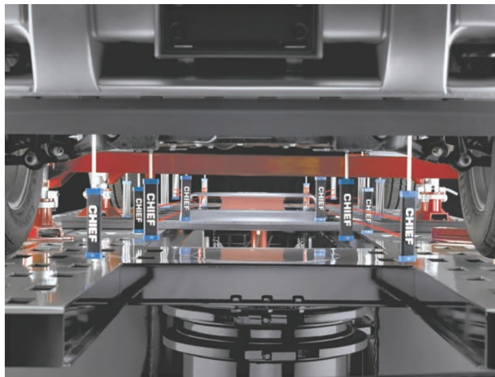
Fig. 5. Positioning of measuring heads and scanning laser during floor plate measurements
