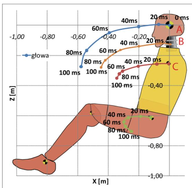
Fig. 4.2. Trajectories of displacement of the characteristic points of the dummy
