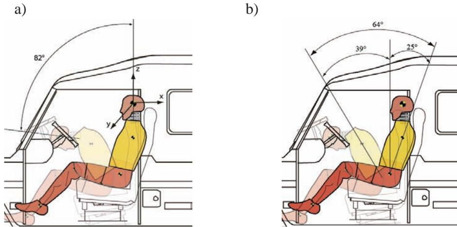
Fig.4.3. Angular displacements of the head (a) and the torso (b); a change of the seat base position resulting from the deformation of the floor along the frame is also shown on the figures
