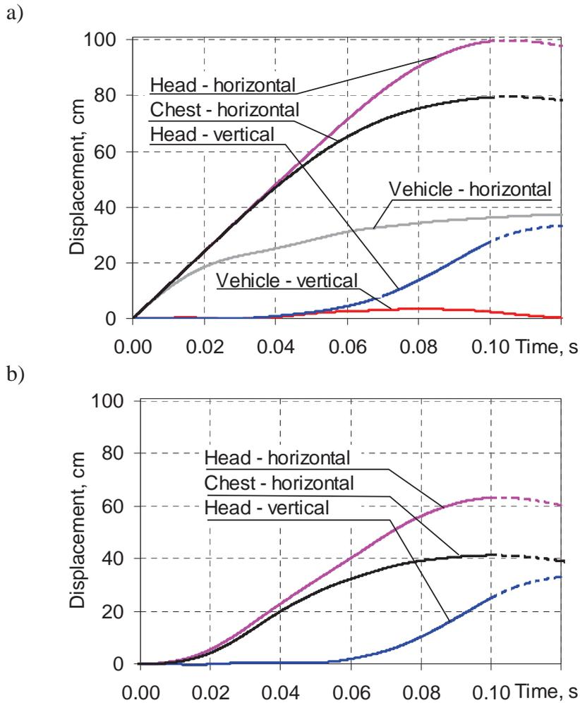
Fig.4.10. Head and chest displacements in relation to the ground (a) and the vehicle (b)
