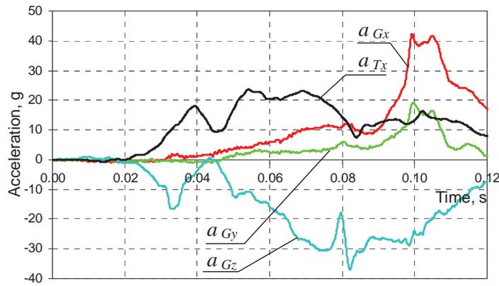
Fig.4.5. Head acceleration realizations, components:  $a_{Gx}$ ,  $a_{Gy}$ ,  $a_{Gz}$  and the component  $a_{Tx}$  of the torso acceleration
