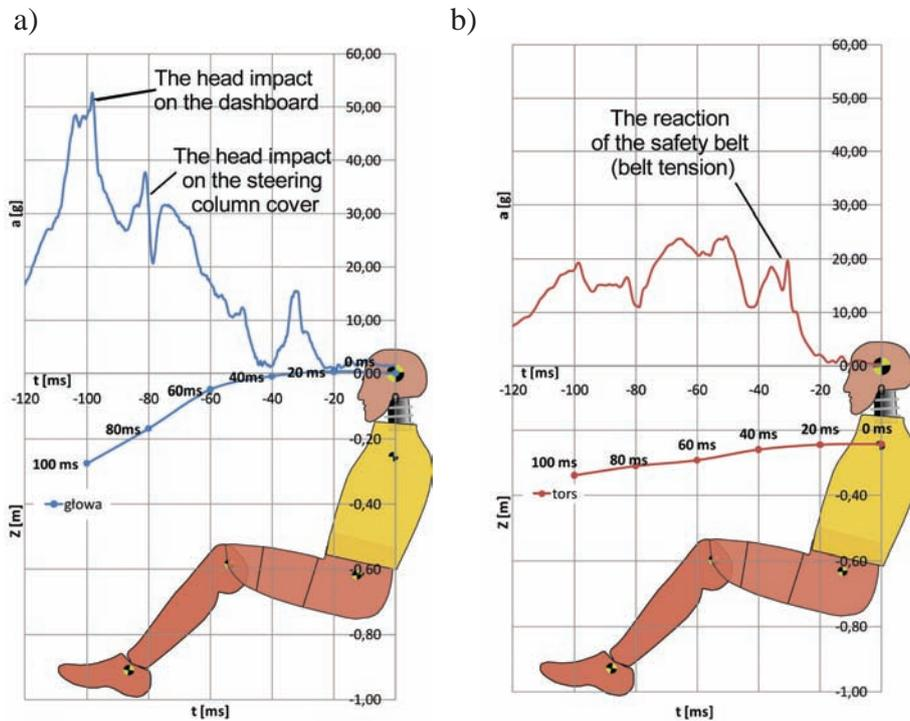
Fig. 4.4. Association of the course of changes of the accident acceleration and the dummy displacement in barrier impact at the speed of 43 km/h; a - the head, b - the torso
