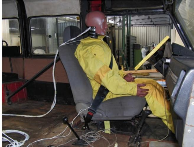
Fig. 2.4. Arrangement of a dummy with sensors during preparation for the tests
