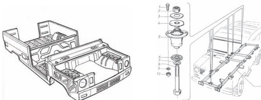
Fig. 2.2. Chassis and its fixing to the longitudinal frame of a vehicle
