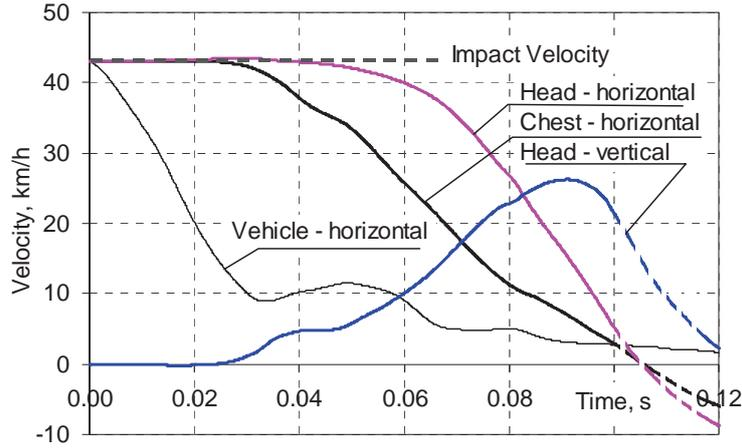
Fig. 4.9. Association of head, torso and cab velocity realization in relation to the ground
