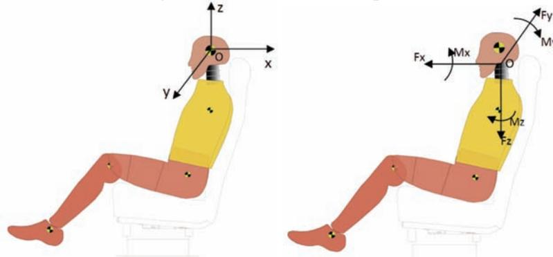
Fig. 2.5. Directions of the acceleration sensor axis in the head and crushing force and moment sensor axis in the neck (initial status)
