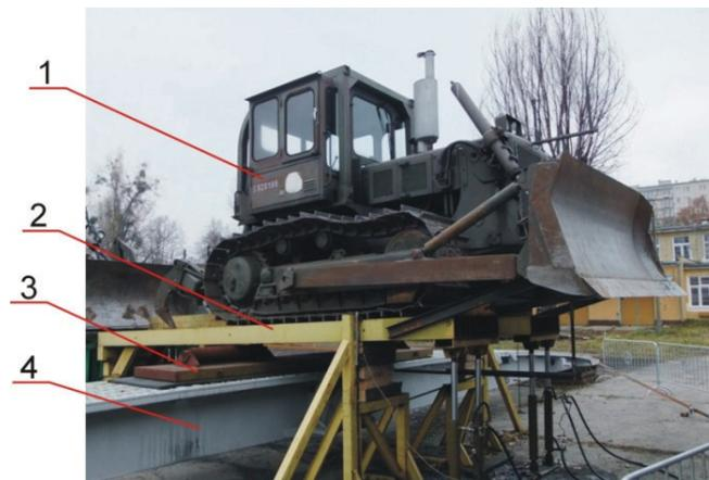
Fig. 6. General view of research stand during test: 1 – load-generating vehicle (SG 15 bulldozer), 2 – loading platform, 3 – load-transfer slab, 4 – BLG-60M2 (BLG67-M2) span (bridge track)
