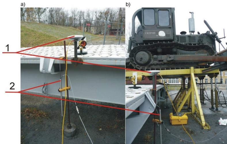
Fig. 8. Measurement arrangement of bridge span deflection curve: 1- antenna for GNSS measurement; 2-inductive displacement sensor a) measurement point no. 1; b) side view of the stand
