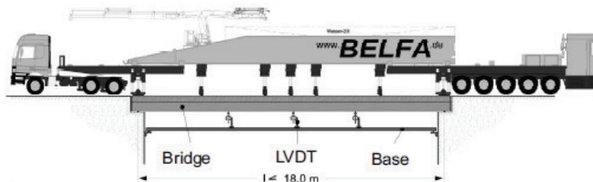
Fig. 4. BELFA truck during span test
