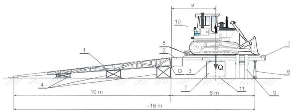
Fig. 5. Diagram of research stand for testing load capacity of bridge tracks: 1 – approach ramp, 2 – loading platform, 3 – load transfer slab, 4 – supports, 5 – front beam, 6 – span-loading actuators, 7 – span (bridge track), 8 – rear beam, 9 – side guides, 10 – load-generating vehicle; 11 – span support
