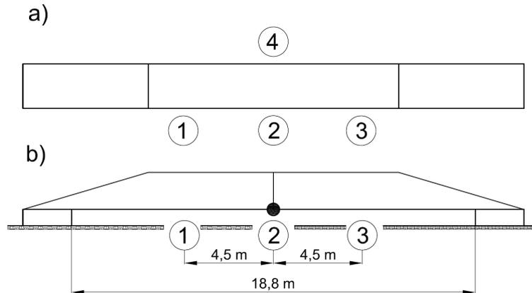
Fig. 7. Diagram showing distribution of measurement points during tests of BLG-60M2 (BLG-67M2) bridge tracks: a) top view, b) side view
