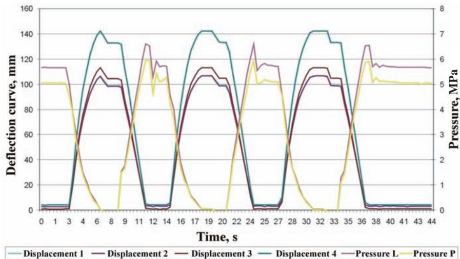
Fig. 9. Timing of changes in deflection curve values and in pressure values inside lifting actuators during one of loading cycles of BLG-60M2 (BLG-67M2) bridge span
