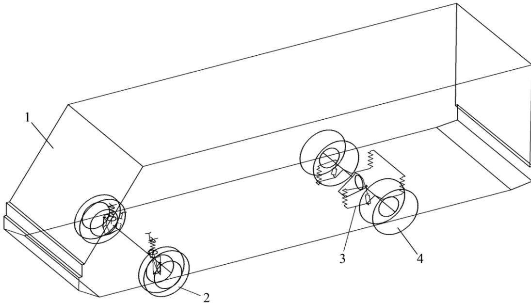
Fig. 2. The General view of the settlement scheme of the bus: 1 – a body, 2 – a forward wheel, 3 – a rear axle, 4 – a back wheel
