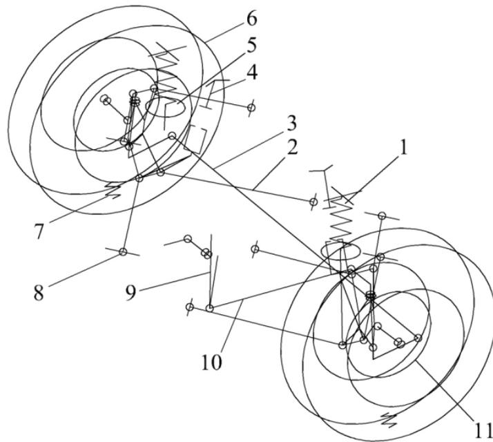
Fig. 3. The front suspension: 1 - an air spring, 2 - the lever, 3 - a cross-section track rod, 4 - the hydraulic shock absorber, 5 - a swivel member, 6 - a front wheel, 7 - the tire, 8 - the hinge; 9 - drop arm, 10 - drag link, 11 - a nave
