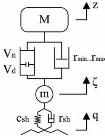
Fig. 1. One-basic two-mass model of a suspension with a controllable damper and a controllable pneumatic spring:  $M, m$  – cushioned and uncushioned masses,  $Z, \zeta$  – vertical displacement of cushioned and uncushioned masses;  $q$  – kinematic fluctuation,  $c_{sh}, r_{sh}$  – rigidity and coefficient of resistance of the tyre,  $V_o, V_d$  – the basic and additional volumes of the pneumatic spring,  $r_{min}, r_{max}$  – the min and max values of damper resistance coefficient
