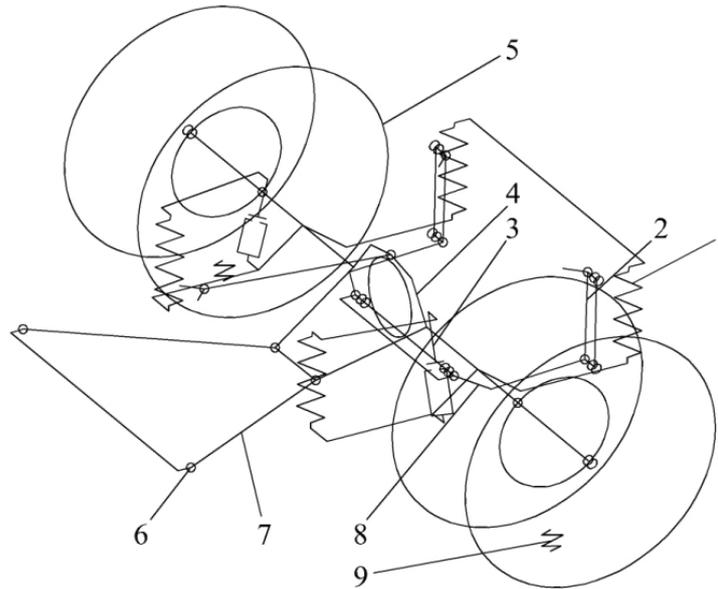
Fig. 4. The rear suspension: 1 - an air spring, 2 - an earring, 3 - the hydraulic shock absorber, 4 - the rear axle, 5 - a rear wheel, 6 - the hinge, 7 - pull-rod, 8 - the antiroll bar, 9 - the tire
