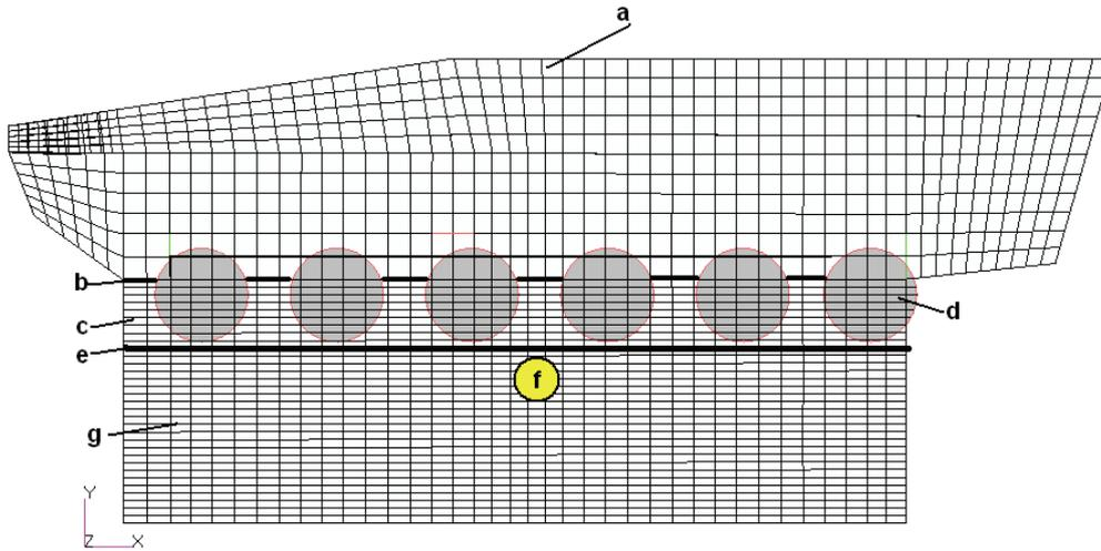
Fig. 6. Scheme of analyzed vehicle: a – hull, b – ALE coupling surface, c – air area, d – wheels, e – border of two domains, g – ground, f – explosive
