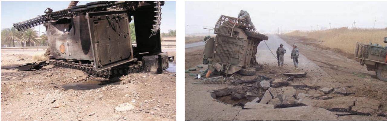
*Fig. 1. An example of IED detonation under different vehicles [US ARMY photo]*
