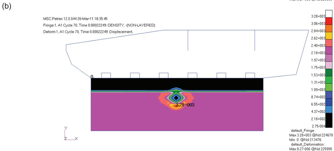
Fig. 8. Pressure distribution trough section of the vehicle (a), ground and air density (b) for the time  $t = 0.00022$  s
