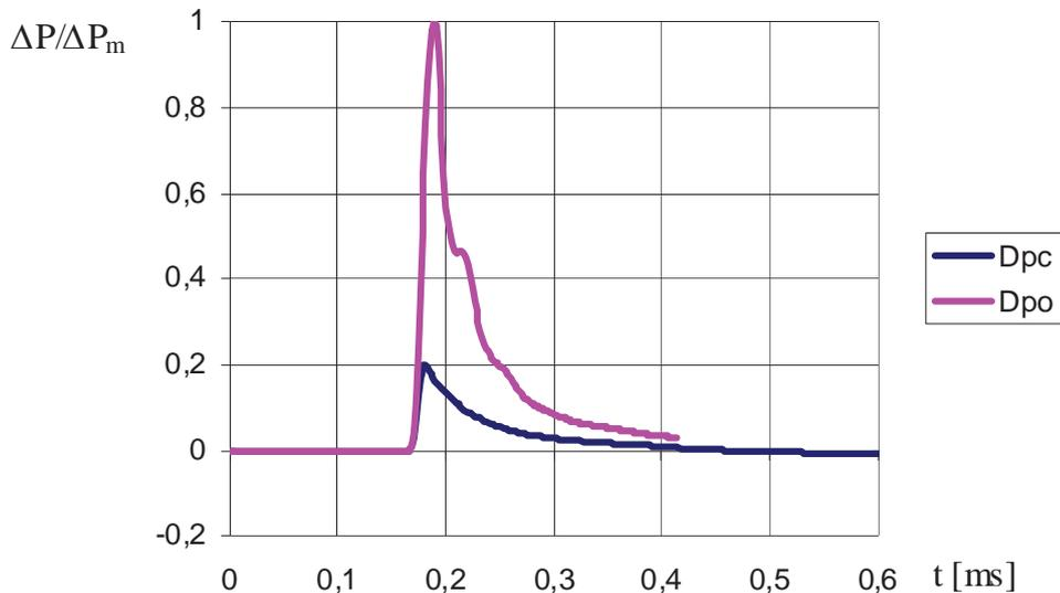
Fig. 4. Comparison of pressure impulse of free wave  $D_{pc}$  and reflected wave  $D_{po}$  for 125 g TNT charge
