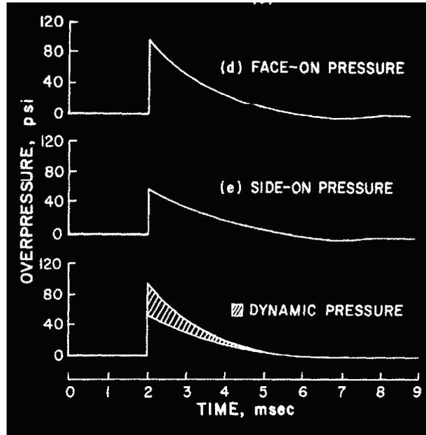
Fig. 3. Static and dynamic pressure for near ground explosion [D. R. Richmond 1970]
