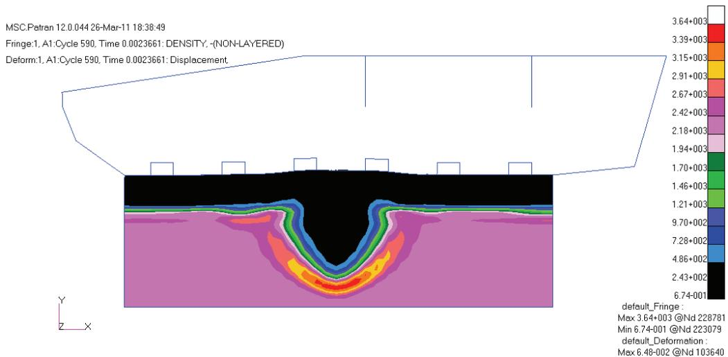
Fig. 10. Pressure distribution trough the symmetry plane section of the for the time  $t = 0.00236$  s
