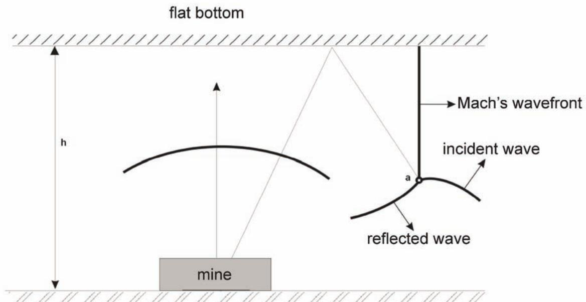
*Fig. 2. Wave reflection from vehicle's bottom*
