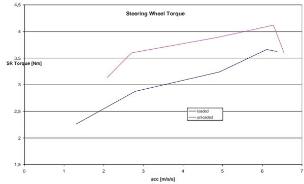
Fig. 4. Steering Wheel Torque (SR Torq) in Lateral Acceleration Function
