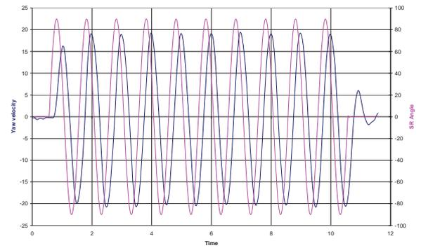
Fig. 8. Time Processes of the Steering Wheel Turn Angle and the Angular Yaw Velocity
