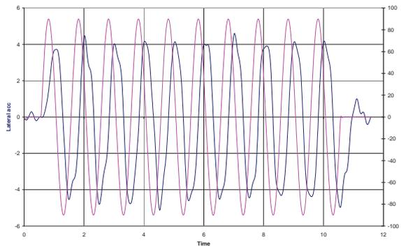
Fig. 7. Time Processes of Steering Wheel Turn Angle and Lateral Acceleration
