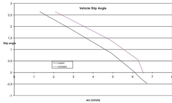
Fig. 5. Vehicle Slip Angle in Lateral Acceleration Function
