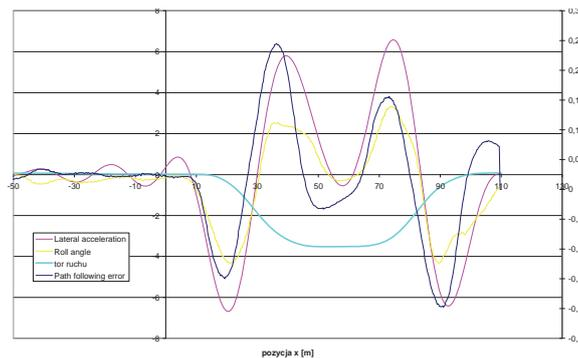
Fig. 13. Time processes of parameters measured during the double-lane-change manoeuvre
