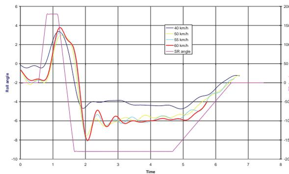
Fig. 12. Time processes of the lateral roll angle during the stability test
