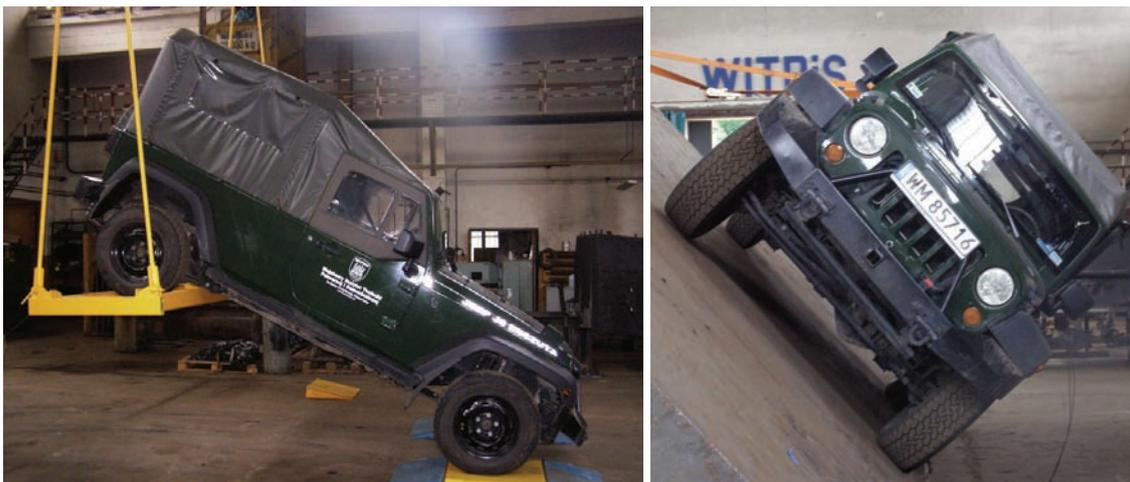
*Fig. 2. Determination of the Centre-of-Mass Position and the Lateral Roll Static Angle*
