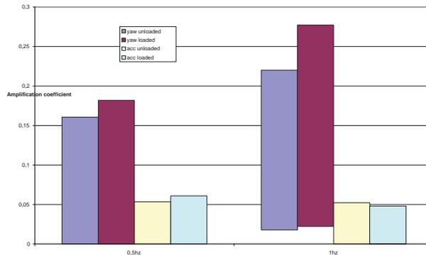
Fig. 11. Amplification coefficients of the lateral acceleration and the angular yaw velocity
