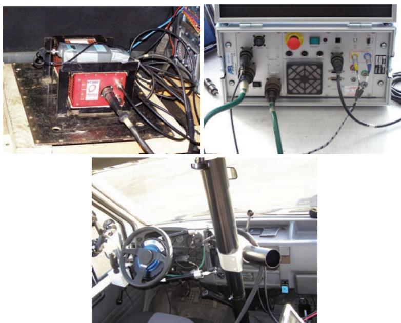
Fig. 1. Steering Robot. a. lag-satellite system RT 3002, b. central unit, c. measurement steering wheel with adjusting pillar
