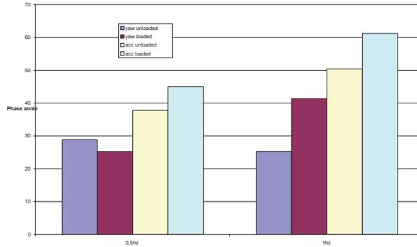
Fig. 10. Phase transition angle between extortion and response of the system
