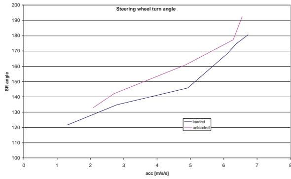
Fig. 3. Steering wheel turn angle, required for driving on a radius of 30 m in the lateral acceleration function
