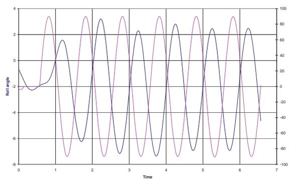
Fig. 9. Time Processes of the Steering Wheel Turn Angle and the Body Roll Angle
