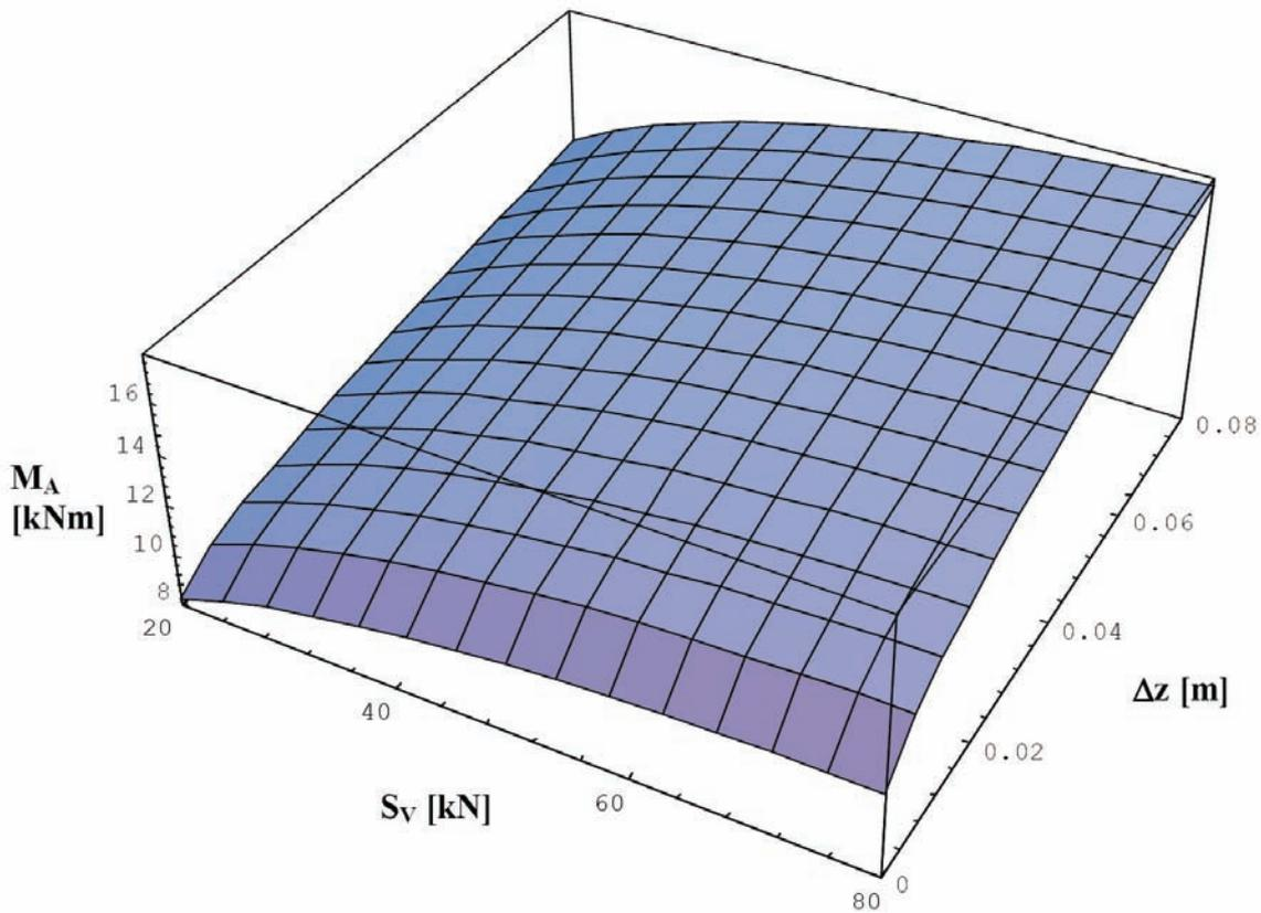
Fig. 8. Driving moment as function of drive pulley sinkage and force in a tension device [2]
