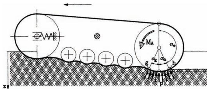
Fig. 1. Track undercarriage on the deformable ground [3]
