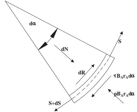
Fig. 7. Distribution of pressures acting on the track element from the tangential area of a drive pulley with deformed ground [2]
