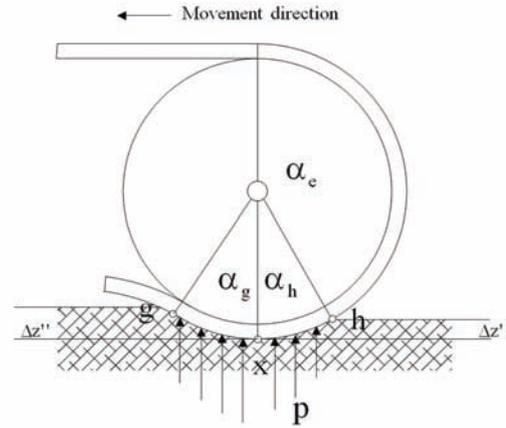
Fig. 5. Interaction of a drive pulley and elastomeric track with pressures on deformable ground ( $\alpha_e$  – wrap range without ground impact,  $\alpha_g$  – additional wrap resulting from ground deformation through a drive pulley,  $\alpha_h$  – wrap range with relaxation of the soil)[2]
