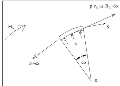
Fig. 2. The forces acting on a separate element of track [2]
