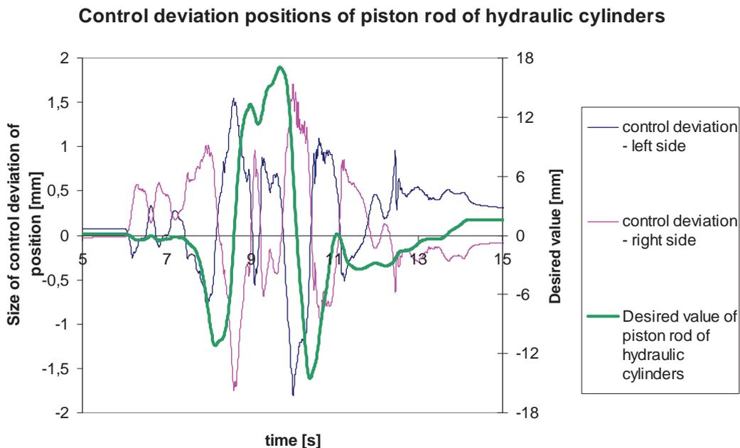
Fig. 4. Test VDA ISO TR 3888 on the testing bench – control deviation positions of piston rod of hydraulic cylinders for supposed speed 60 km/h, sampling rate for control system 100 Hz, load for wheels 4.5 kN, tyres 15”
