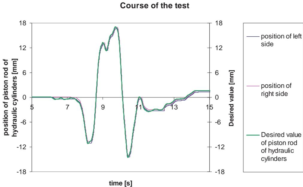
Fig. 3. Test VDA ISO TR 3888 on the testing bench - position of piston rod of hydraulic cylinders for supposed speed 60 km/h, sampling rate for control system 100 Hz, load for wheels 4.5 kN, tyres 15”
