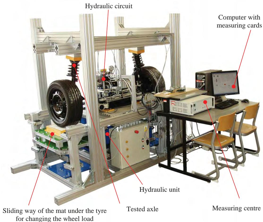
Fig. 2. View of the testing bench for the testing of steering at zero angular speed of wheels
