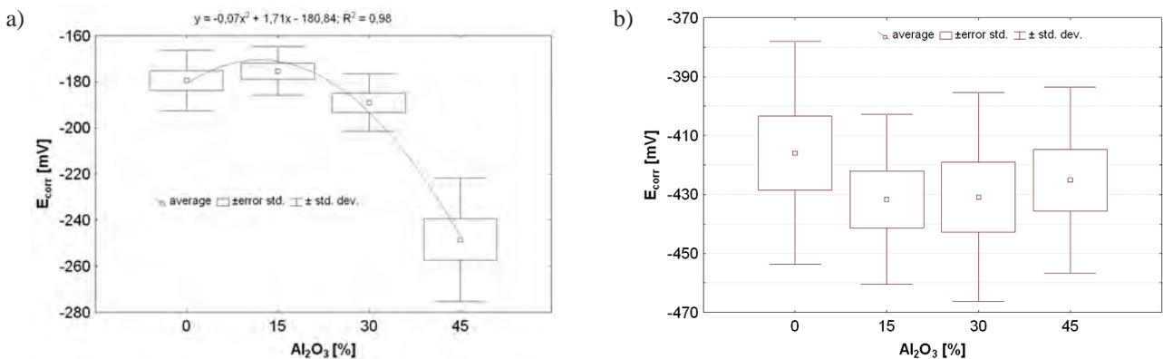
Fig. 3. The alumina oxide influence on corrosion potential values  $E_{corr}$  coatings in a) 0.01 M H<sub>2</sub>SO<sub>4</sub> and b) 3.5% NaCl environments
