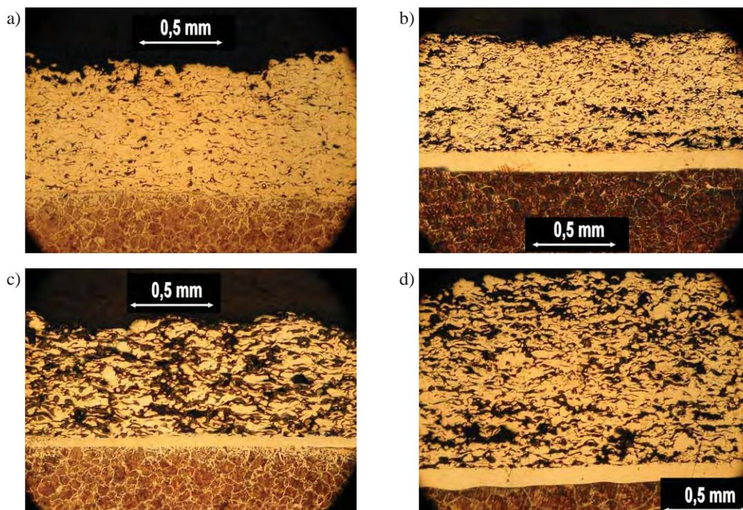
Fig. 1. The structure of flame spraying coatings obtained by “Casto-Dyn 8000” torch: a) Ni-5%Al, b) Ni-5%Al-15%Al<sub>2</sub>O<sub>3</sub>, c) Ni-5%Al-30%Al<sub>2</sub>O<sub>3</sub>, d) Ni-5%Al-45%Al<sub>2</sub>O<sub>3</sub>
