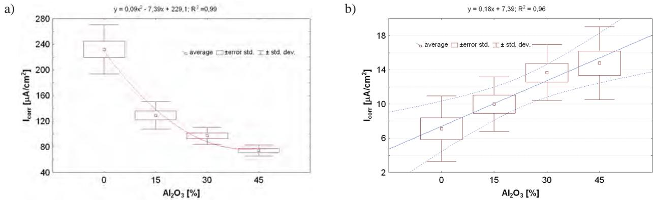
Fig. 4. The alumina oxide influence on corrosion current density values  $I_{corr}$  coatings in a) 0.01 M  $\text{H}_2\text{SO}_4$  and b) 3.5% NaCl environments
