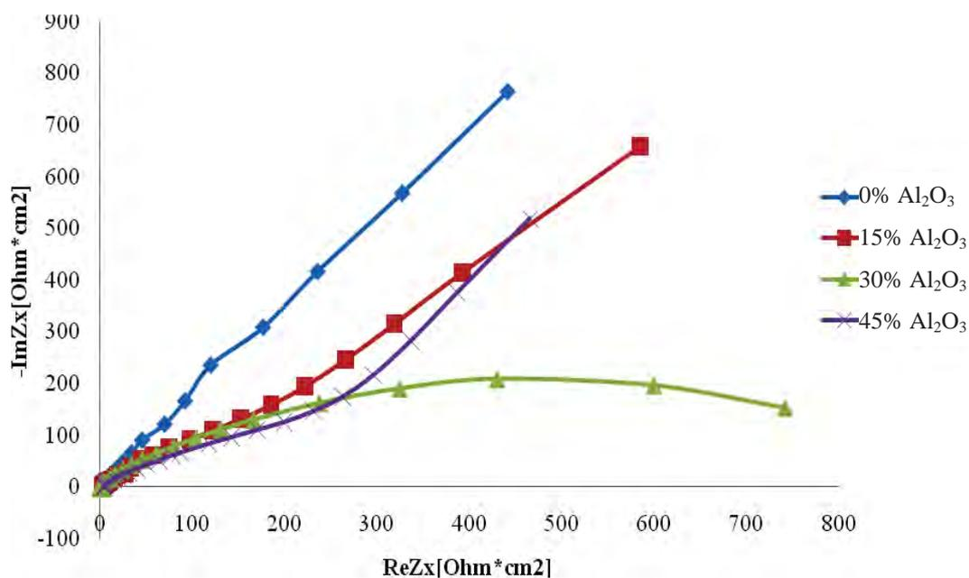
Fig. 5. The samples of impedance spectra of coatings in 3.5% NaCl environment
