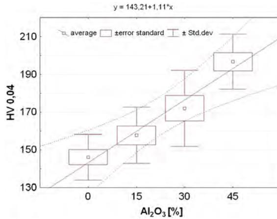
Fig. 2. The microhardness of Ni-5%Al alloys and Ni-5%Al-Al<sub>2</sub>O<sub>2</sub> composites coating obtained by “Casto-Dyn 8000” torch
