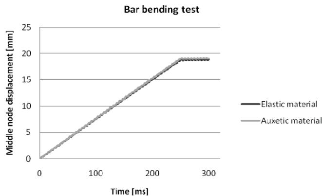
Fig. 3. Bending test deflection / time curve
