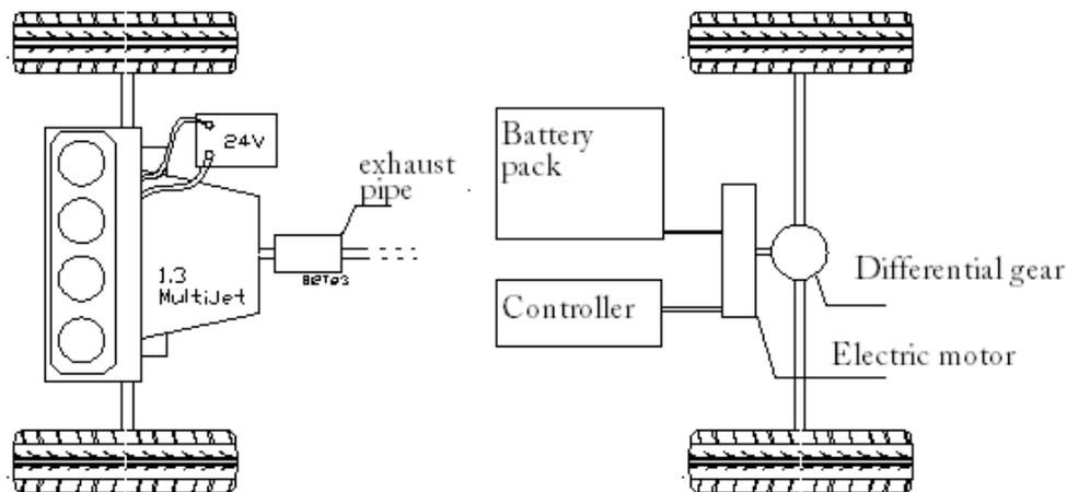
Fig. 1. Prototype hybrid powertrain layout
