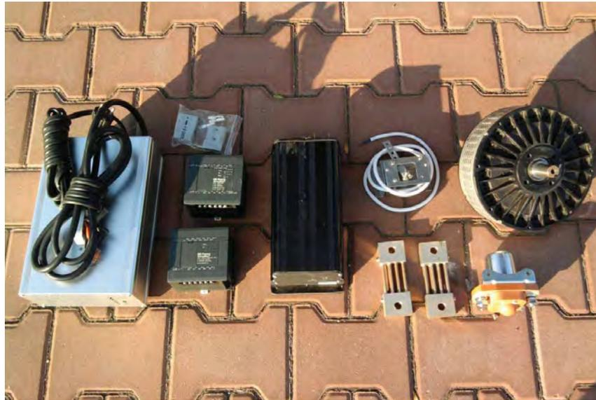
Fig. 4. Electric components of the hybrid powertrain
