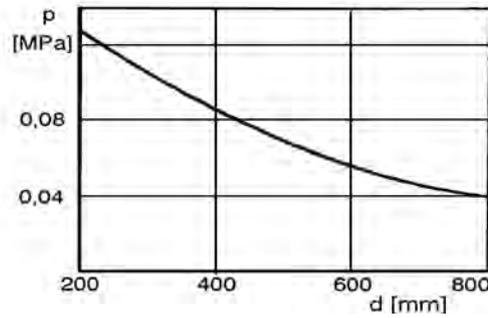
Fig. 6. Change of compression ring mean pressure in low-speed engines [10]
