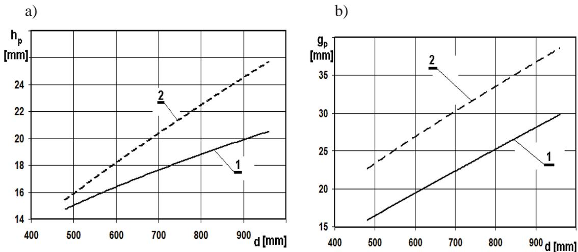
Fig. 3. Relations between ring diameter  $d$  and its: a – axial height  $h_p$ ; b – radial thickness  $g_p$ ; presented results have been achieved for a group of marine engine piston rings: modern – 1 (continuous line), previous – 2 (dashed line)
