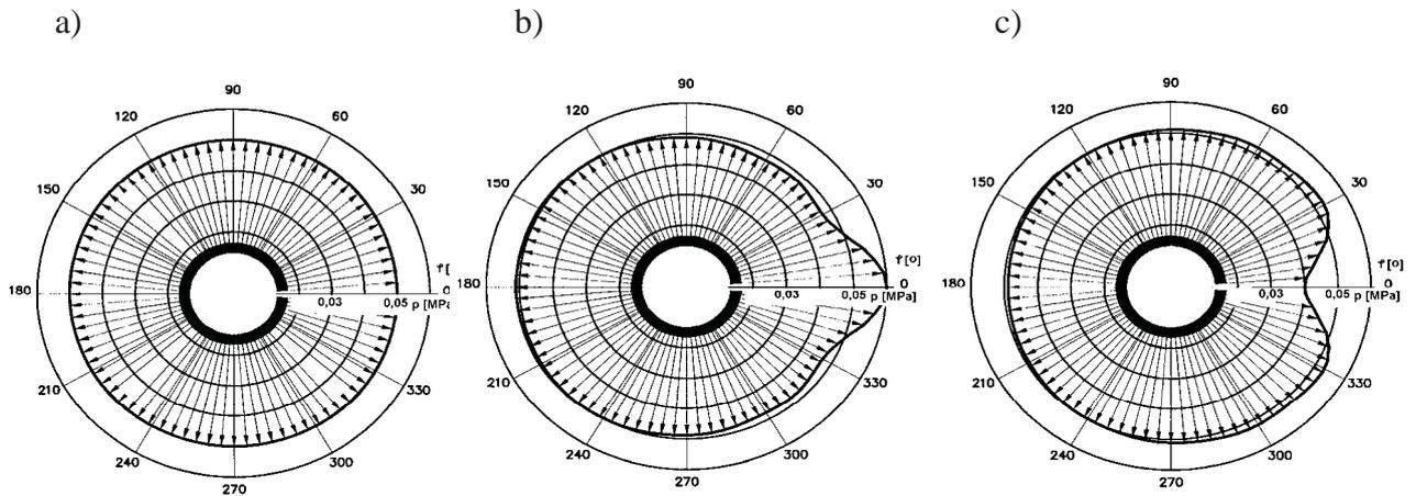
Fig. 8. Exemplary ring to bore pressure distribution; a – even pressure, b – pressure higher in the vicinity of joint, c – pressure lowered in the vicinity of joint; mean pressure  $p = 0.05 \text{ MPa}$
