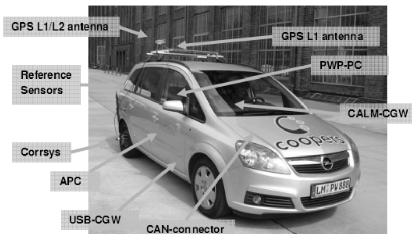
Fig. 3. PWP concept car with COOPERS OBU and independent reference system
