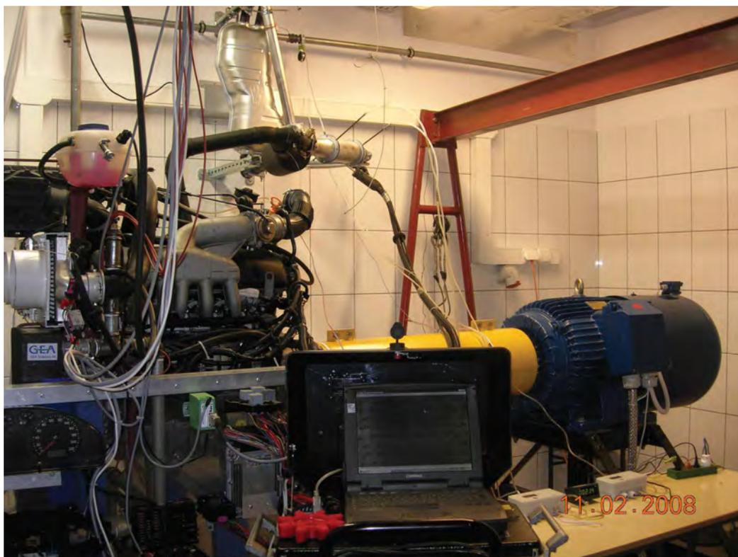
*Fig. 3. Engine test stand*
