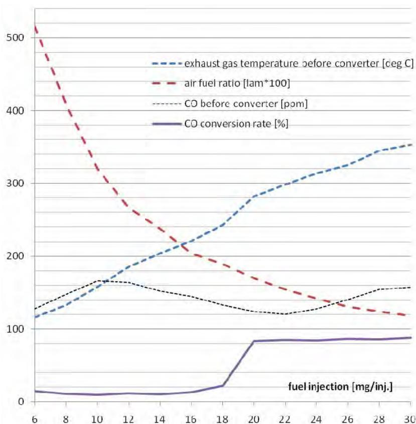
Fig. 4. The influence of exhaust gases temperature on the conversion of the nanotube converter
