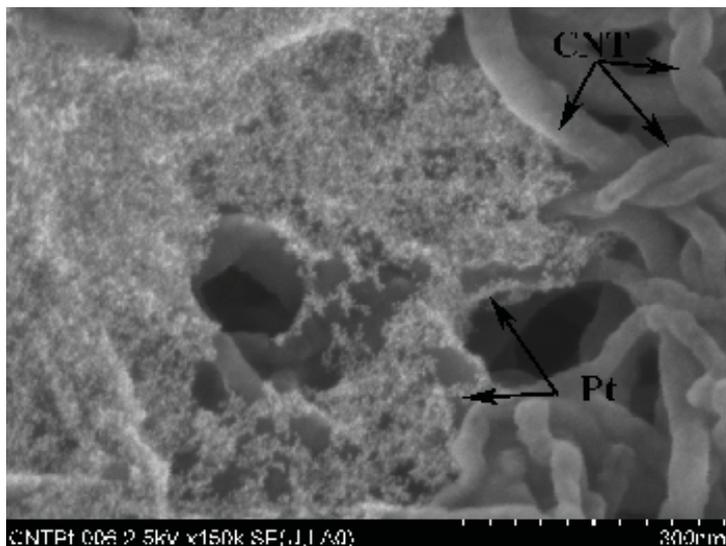
*Fig. 2. Carbon nanotubes covered with nanoparticles of platinum. Real picture of the pre-prototype contact surface with exhaust gases obtained by means of a transmission electron microscope*
