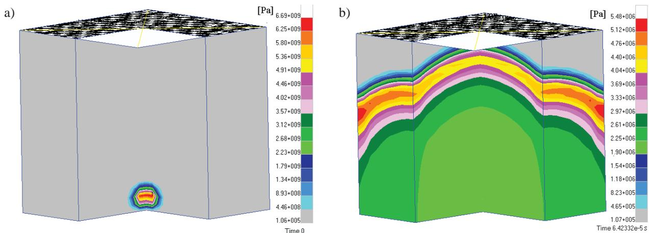
Fig. 2. A view of the pressure wave for two moments of time a) 0 s, b)  $6.4233E-5s$
