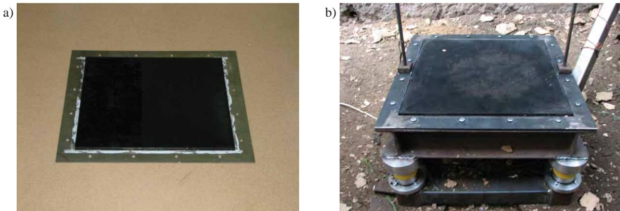
Fig. 11. Object 2: a) a 2 mm thick plate with an elastomer layer; b) deformation obtained from the experiment
