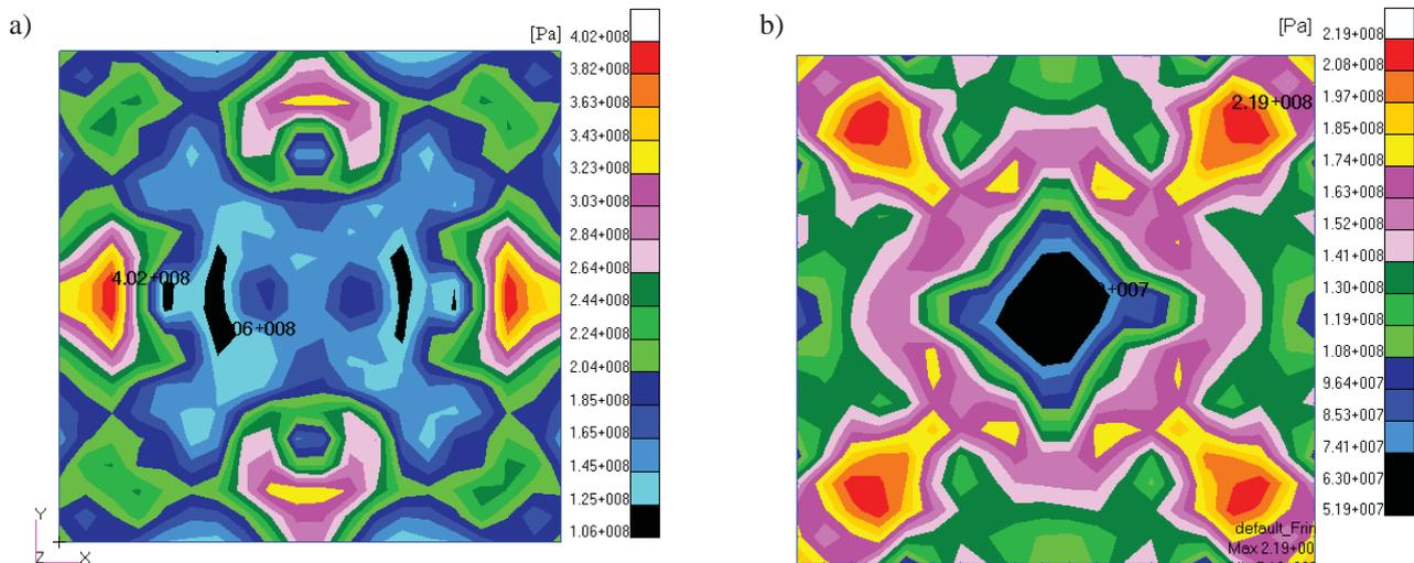
Fig. 6. Comparison of equivalent stress maps for model 1 and 2, a – model 1, b – model 2
