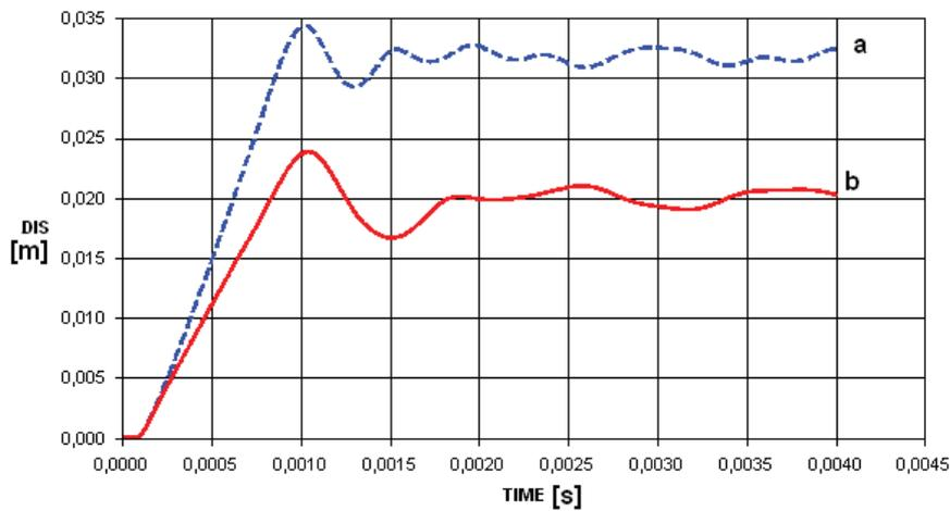
Fig. 4. Displacements of the central node of the metal plate in the function of time, a – model 1, b – model 2
