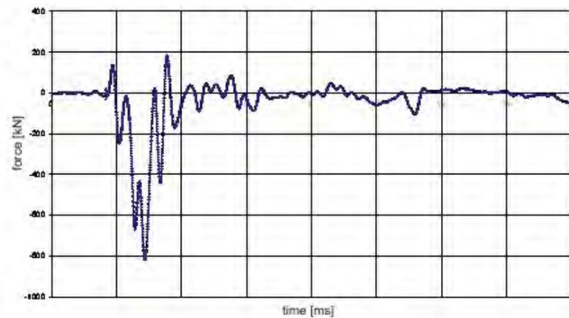
Fig. 9. The course of changing of loading a panel made of steel metal plate with an elastomer layer filled with nanotubes
