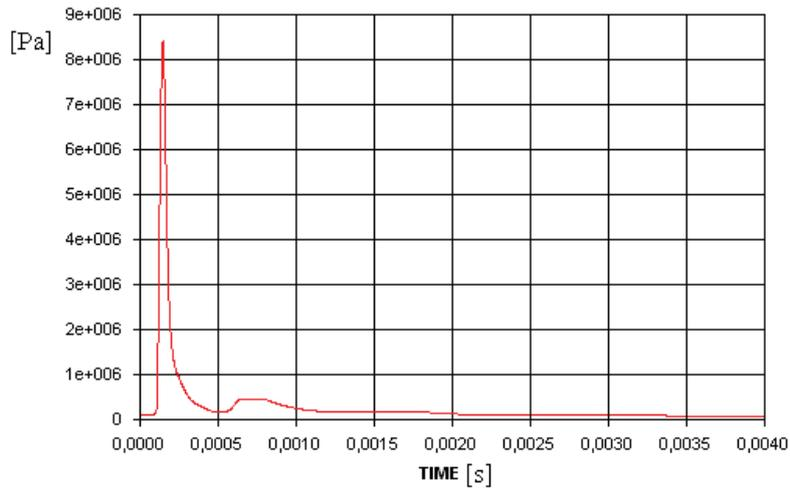
Fig. 3. A blast wave reflected from a 2 mm thick steel sheet metal
