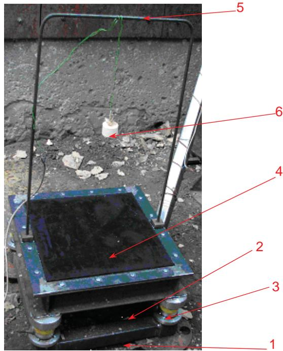
Fig. 7. The system for forces measurement used in the investigations: 1 – a base, 2 – a frame for fixing the panel, 3 – a extensometer force convector (4 items), 4 – an energy absorbing panel, 5 – a frame of fixing the explosive panel, 6 – an explosive material
