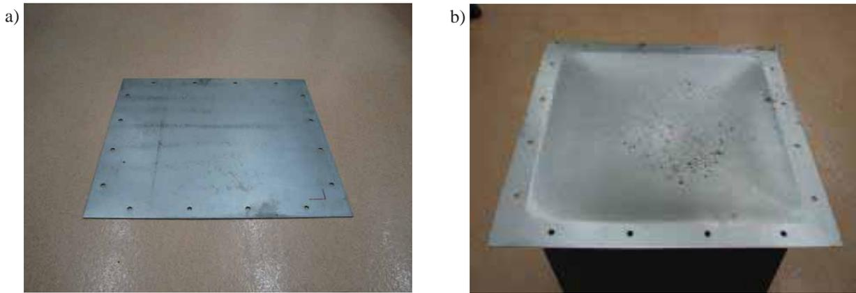
Fig. 10. Object 1: a) a 2 mm thick plate; b) deformation obtained from the experiment
