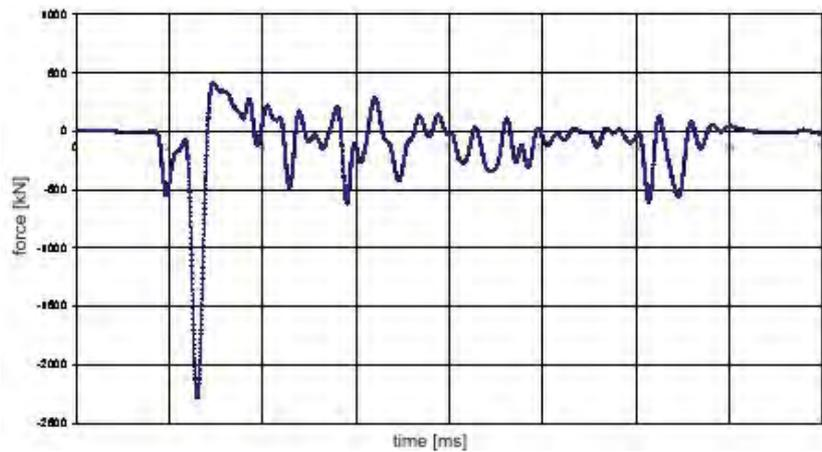
Fig. 8. The course of changes of loading a panel made of steel metal plate
