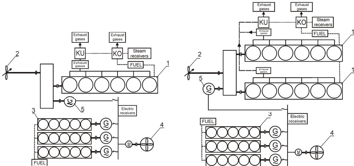
Fig. 3. Marine engine room with shaft generator and controllable pitch propeller driven by medium speed main engine: 1 – main engine, 2 – propeller, 3 – exhaust gas diesel generators, 4 – bow thruster, 5 – shaft generator, G – generator, M – motor, KU – Exhaust gas boiler, KO – auxiliary fired boiler
