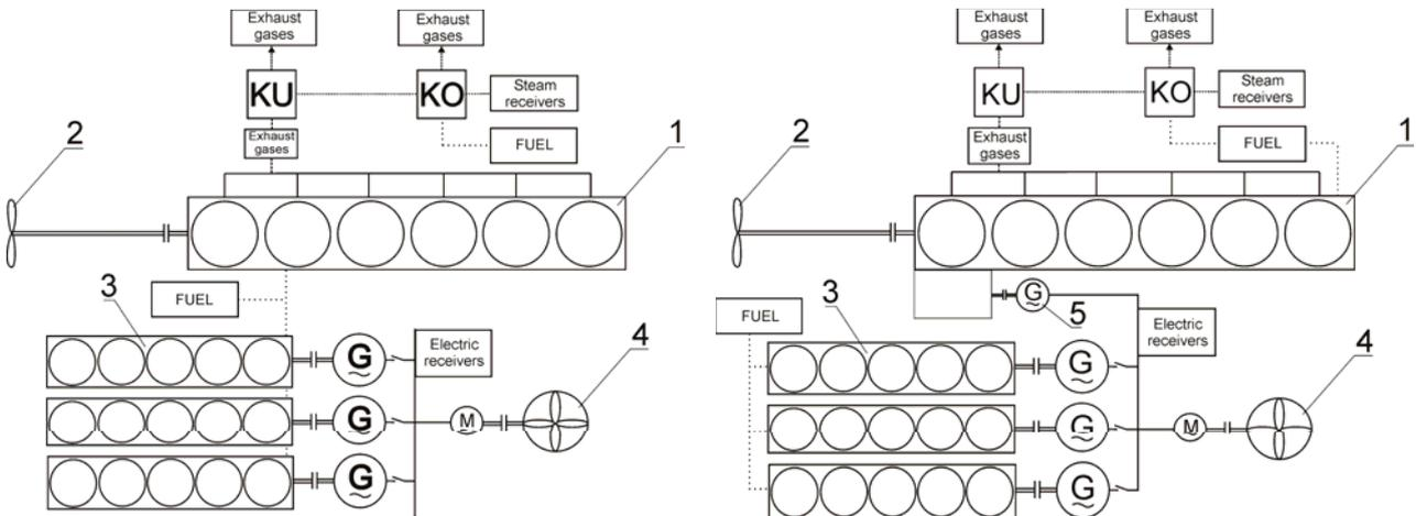
Fig. 2. Marine engine room with fixed pitch propeller driven by two stroke low-speed main engine: 1 – main engine, 2 – propeller, 3 – exhaust gas diesel generators, 4 – bow thruster, 5 – shaft generator, G – generator, M – motor, KU – Exhaust gas boiler, KO – auxiliary fired boiler
