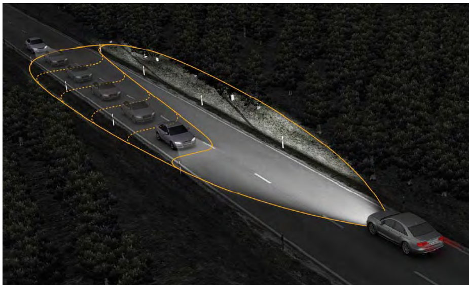
Fig. 2. Audi A8. The passing beam light is automatically reduced by an approaching vehicle [3]
